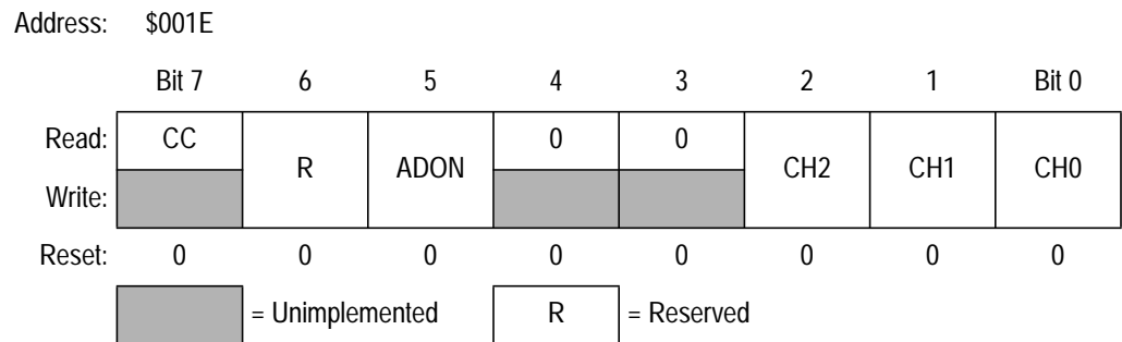
Figure 9-1. A/D Status and Control Register (ADSC)
