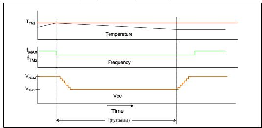
The PROCHOT# signal is asserted when a high temperature situation is detected, regardless of whether Thermal Monitor 1 or Thermal Monitor 2 is enabled.
