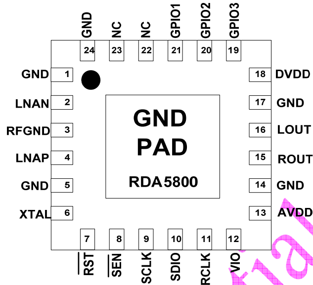
Figure 0-1. RDA5800 Top View
