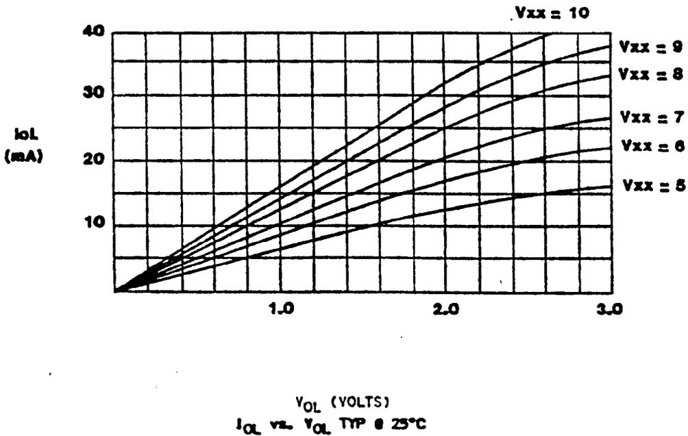
The Output Sink Current is dependent on the  $V_{xx}$  supply and the output load. This chart shows the typical curves used to express the output drive capability.
