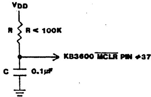
Master Clear requires  $>1.0ms$  delay before activation after power is applied to the  $V_{DD}$  pin. To achieve this, an external RC configuration as shown can be used (assuming  $V_{DD}$  is applied as a step function).
