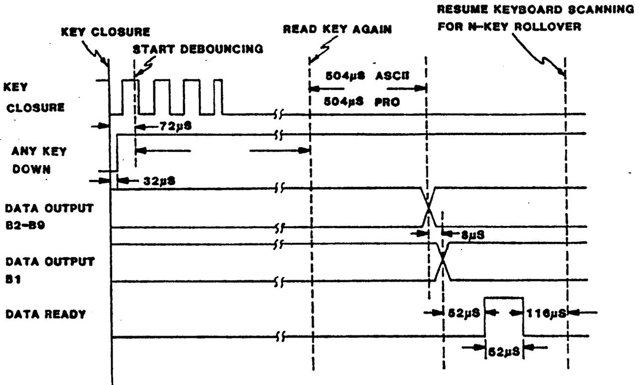
Timing Based on  $T_{CY} = 4 \mu s$  ( $F_{OSS} = 1 MHz$ )
