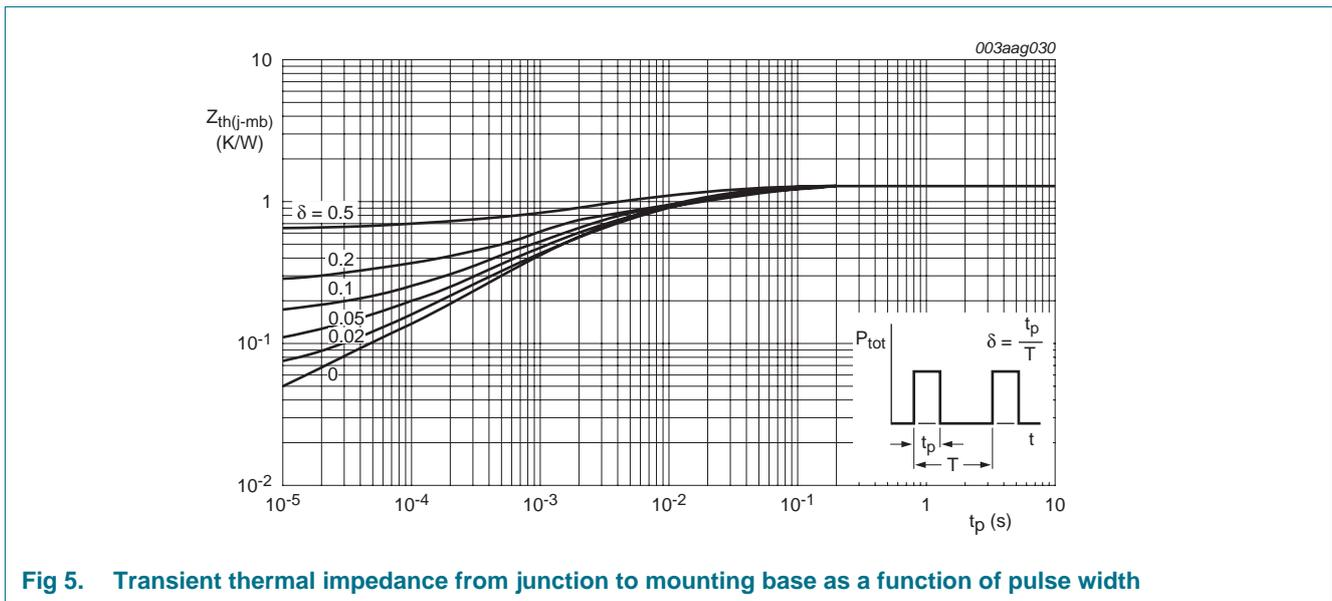
**Fig 5. Transient thermal impedance from junction to mounting base as a function of pulse width**
