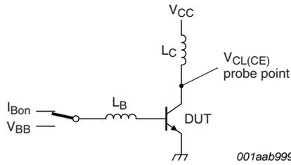
$V_{CL(CE)} \leq 1000 \text{ V}; V_{CC} = 150 \text{ V}; V_{BE} = -5 \text{ V};$
