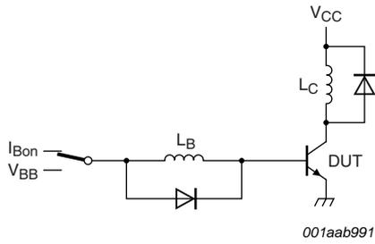
$V_{CC} = 300\text{ V}; V_{BB} = -5\text{ V}; L_C = 200\ \mu\text{H}; L_B = 1\ \mu\text{H}$
