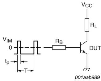
$V_{IM} = -6 \text{ to } +8 \text{ V}; V_{CC} = 250 \text{ V}; t_p = 20 \mu\text{s}; \delta = \frac{t_p}{T} = 0.01$
