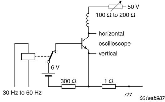
**Fig 6. Test circuit for collector-emitter sustaining voltage**
