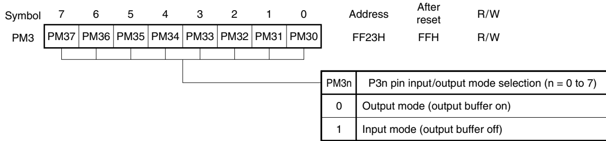
Figure 13-3. Format of Port Mode Register 3
