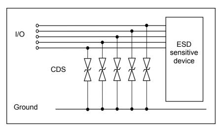
Protection of I/O Lines with discrete CeraDiodes
