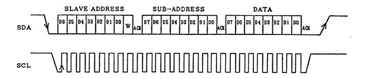
The  $\mu$ PC1852 has auto increment function which increments the subaddress automatically in write mode. (Bit D7 of Subaddress O6H is "1".)
