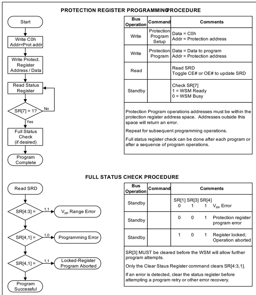
Figure 36. Protection Register Locking
