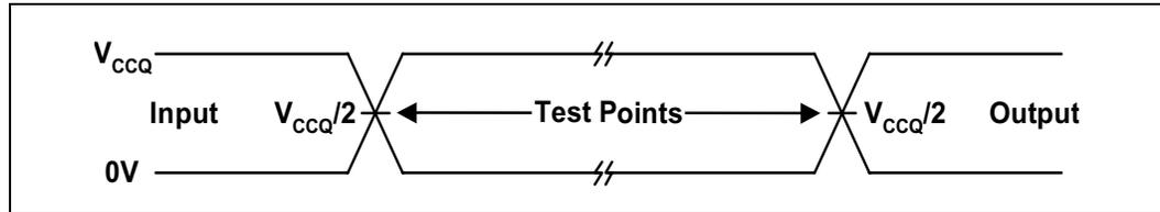
**NOTE:** Input timing begins, and output timing ends, at  $V_{CCQ}/2$ . Input rise and fall times (10% to 90%) < 5 ns. Worst case speed conditions are when  $V_{CC} = V_{CCMin}$ .
