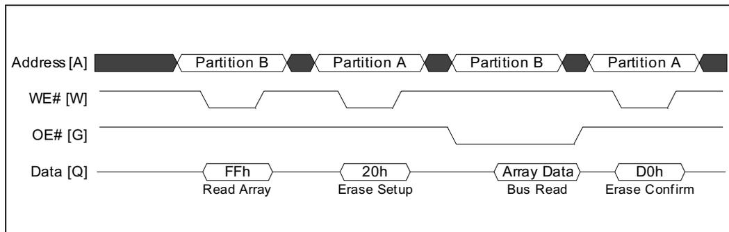
By contrast, a write bus cycle may not interrupt a 2-cycle write sequence. Doing so causes a command sequence error to appear in the status register. [Figure 27](#) illustrates a command sequence error.
