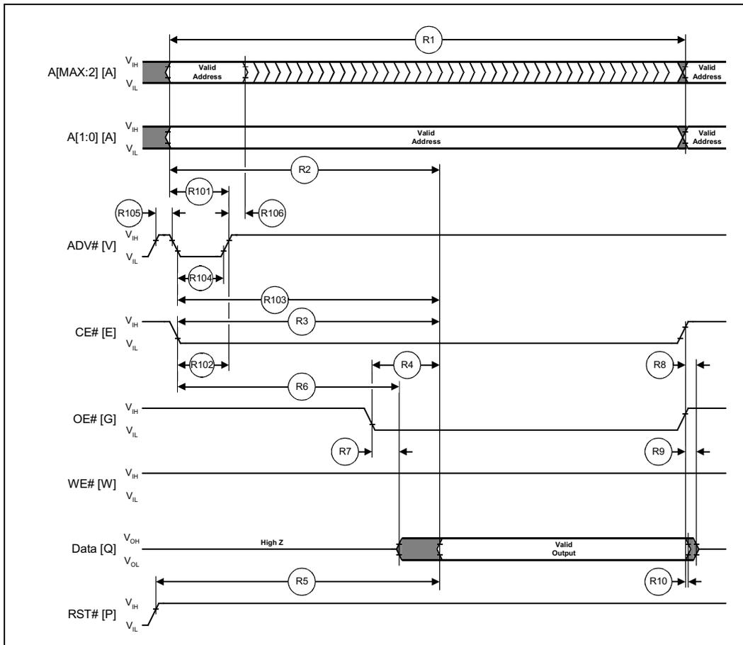
Figure 10. Page-Mode Read Operation Waveform
