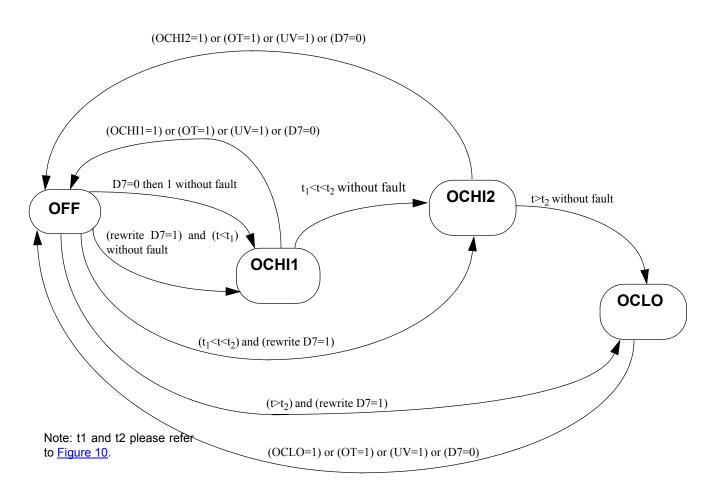
Figure 11. Faults management in Normal Mode (for OUT[1:5] only)
