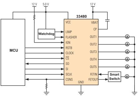
Figure 1. 33480 Simplified Application DiagraM
