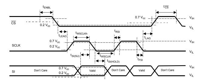
Figure 4. Input Timing Switching Characteristics
