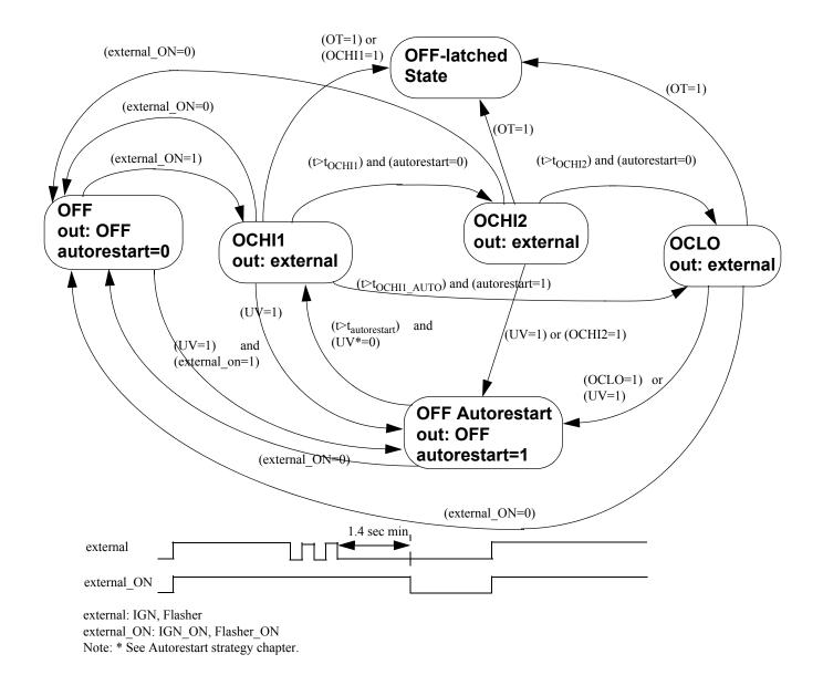
Figure 12. Faults management in Fail Mode (for OUT[1:5] only)
