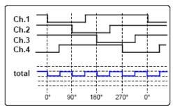
The synchronization of the switching phases between different corner light IC is provided by an SPI command in combination with the  $\overline{CS}$  input. The bit in the SPI is called PWM sync (initialization register).
