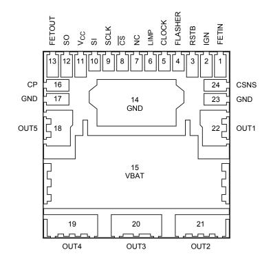
Figure 3. 33480 Terminal Connections (Transparent Top View Of Package)
