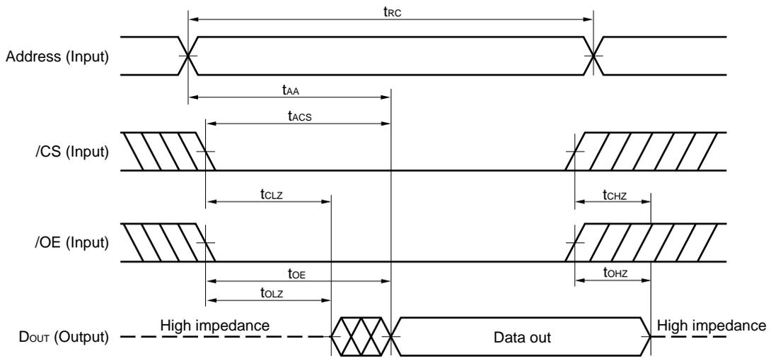
**Caution** Address valid prior to or coincident with /CS low level input.
