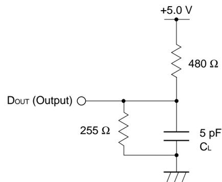
**Remark**  $C_L$  includes capacitances of the probe and jig, and stray capacitances.
