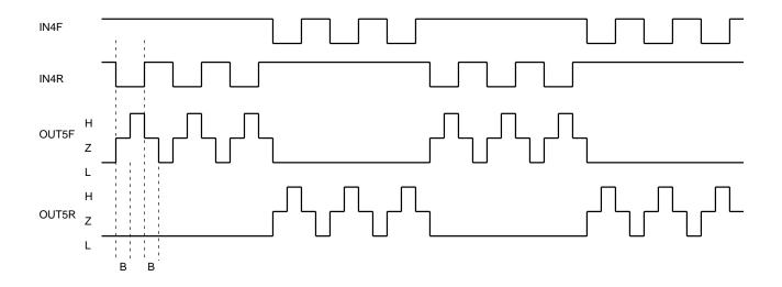
LOADING contains the OFF section B (about  $1\mu s$ ) on both edges for changeover of the input. With the input at HH, the short braking occurs on the lower side.
