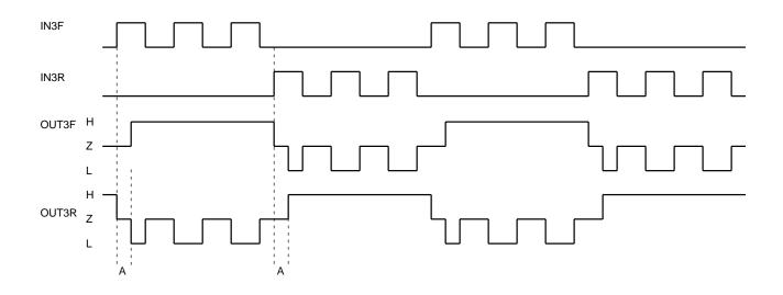
SLED performs PWM on the lower side. In this case, the upper side of another phase is always ON. Only initial changeover contains the OFF section A (about  $1\mu s$ ) as a measure for through operation. OUT4F and R do the same operation.
