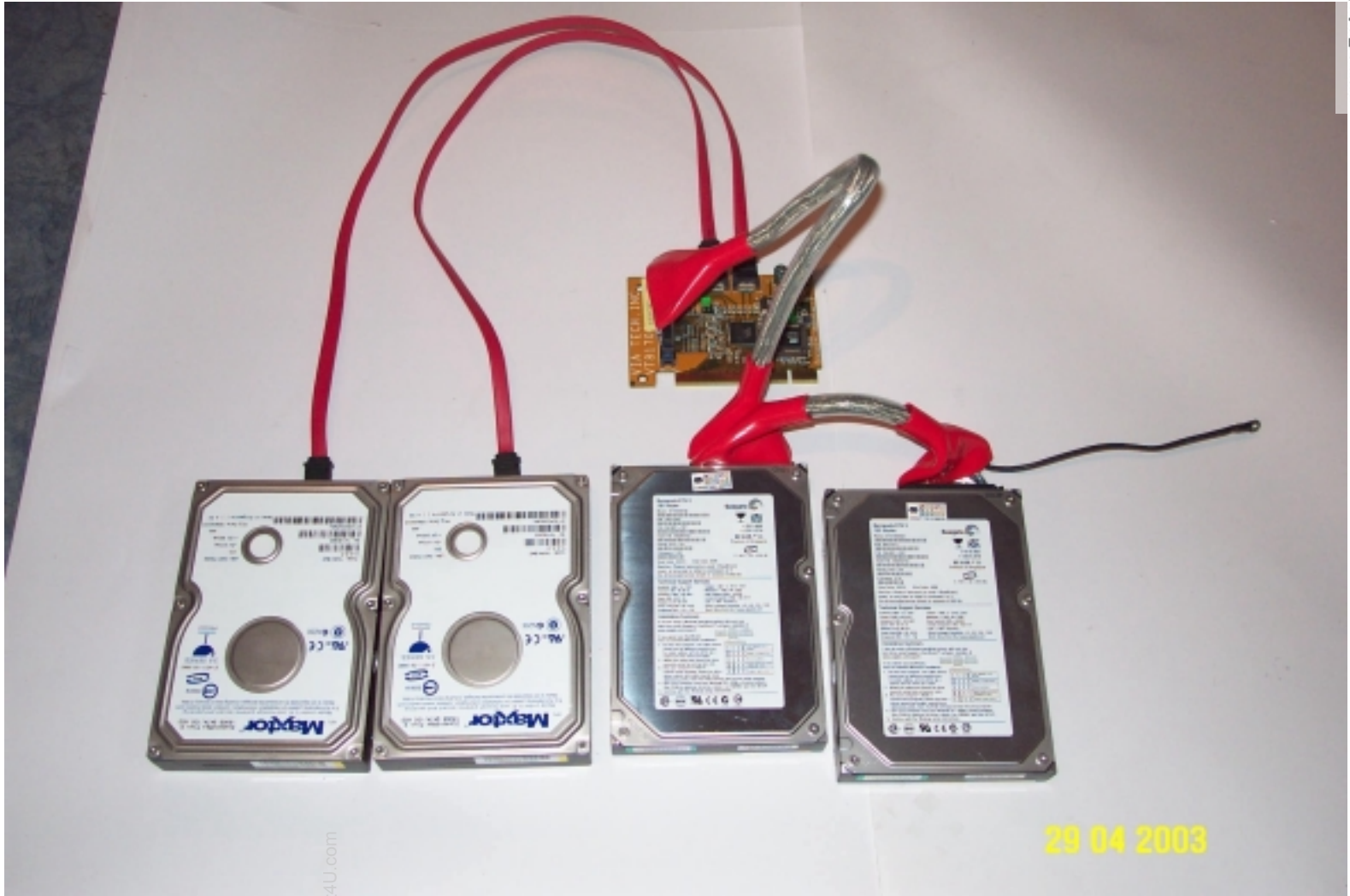
SATA Cabling (left) vs PATA Cabling (right)
