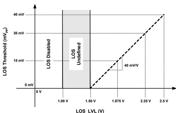
Figure 2. LOS\_LVL Mapping
