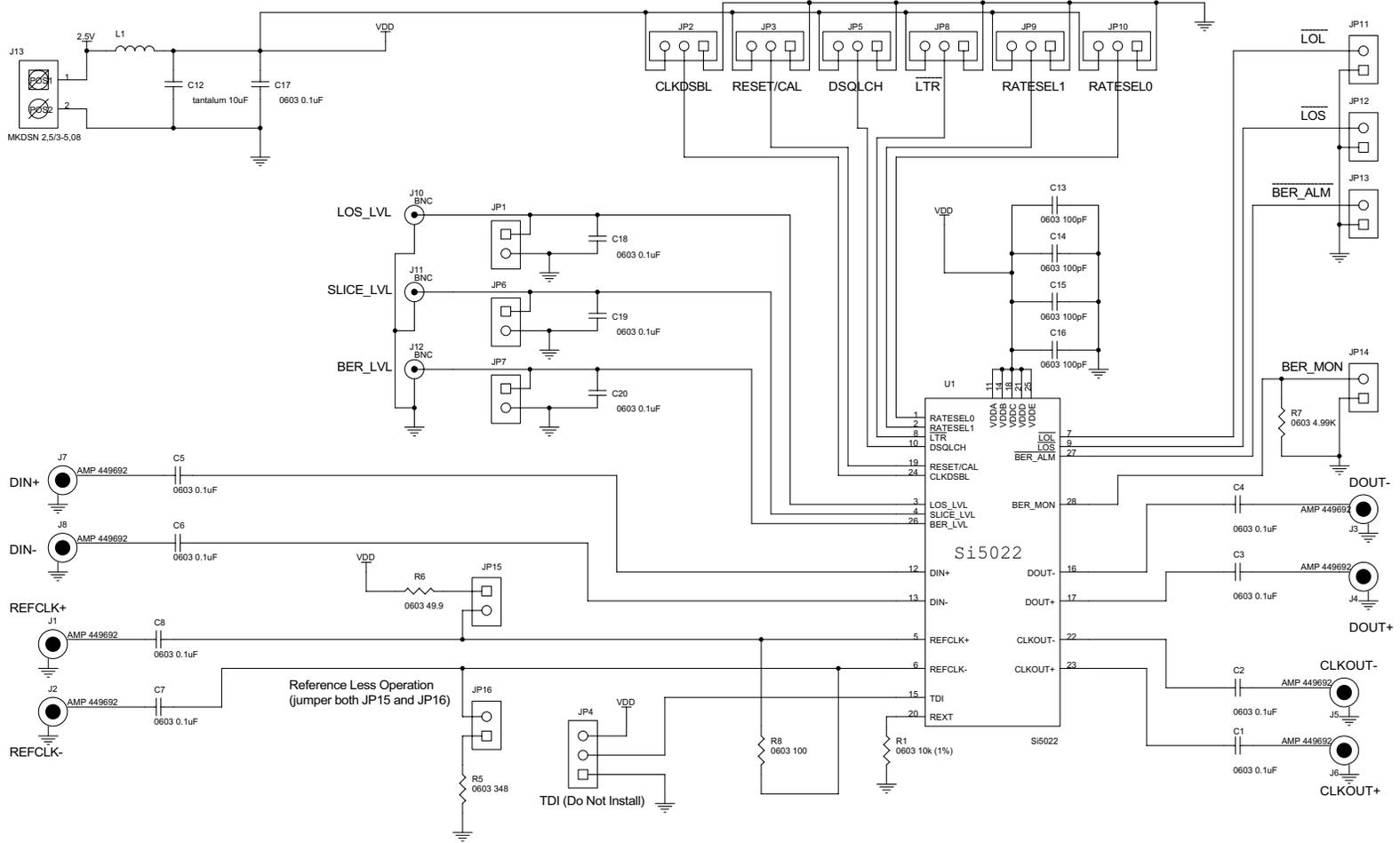
Figure 4. Si5022 Schematic
