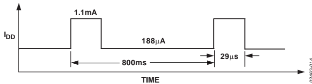
Figure 14. Mode 1 Power Dissipation
