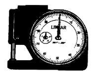
This handy pocket gauge weighs less than two ounces. It is ideal for measuring the thickness of paper, leather, sheet metal, rubber & more. Apvil dia. 5.9mm.
