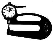
Linear's Dial Thickness Gauge is light in weight, easy to handle and carry. This specially built gauge is mounted in a hand contoured frame with a thumb release mechanism; has fast direct reading to .01mm, measuring range 10mm, throat depth 100mm.
