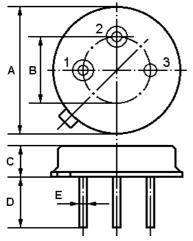
Pin Configuration 1 Input / Output 2 Output / Input 3 Case Ground Dimension Data (unit: mm) 9.30±0.20 A В 5.08±0.10 С 3.40±0.20 D 3±0.20 / 5±0.20 Е 0.45±0.20
