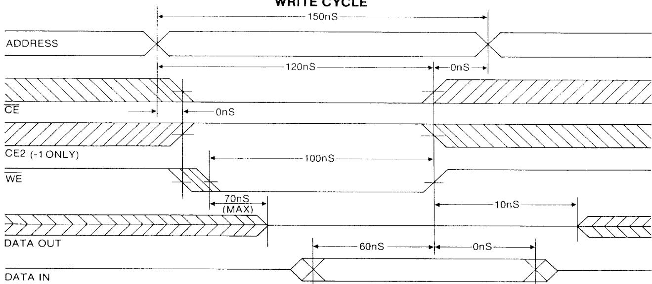
If OE is high during a WE controlled write cycle, the output buffers remain in a high impedance state in this period. Timing measurement reference level is 1.5 volts.
