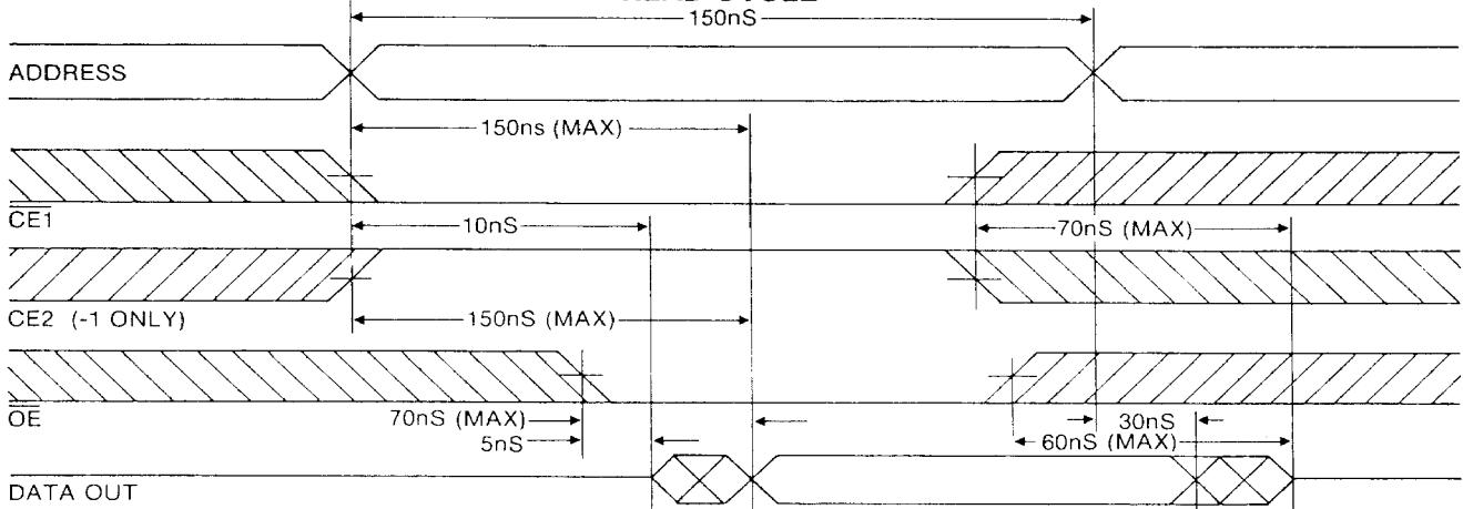
WE is high during read cycle. Timing measurement reference level is 1.5 volts.
