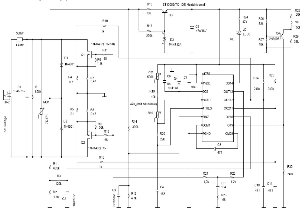
A typical application schematic for a 350W load.
