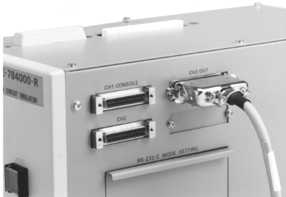
Photo 2-7 Connecting PC Bus Interface Cable
