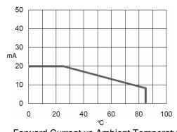
Forward Current vs Ambient Temperature
