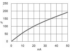
Relative Luminous Intensity vs Forward Current
