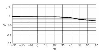
Relative Luminous Intensity vs Ambient Temperature
