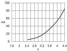
Forward Current vs Forward Voltage
