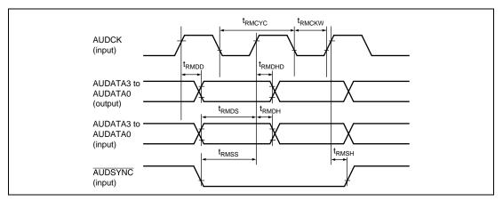
Figure 26.29 RAM Monitor Timing
