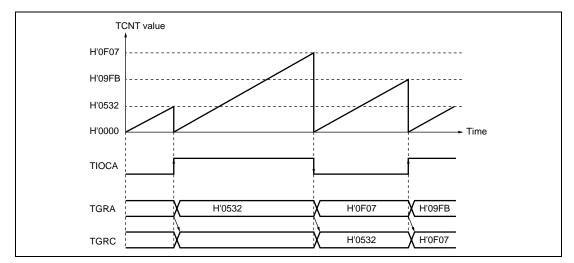
Figure 11.17 Example of Buffer Operation (2)
