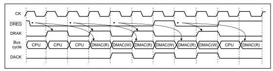
Figure 10.18 Burst Mode, Dual Address and Level Detection (Fastest Operation)
