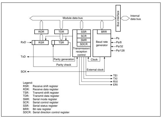
Figure 13.1 Block Diagram of SCI
