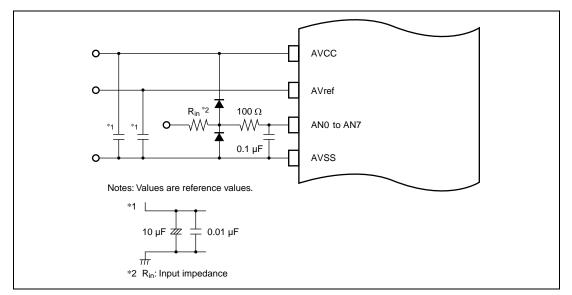
Figure 15.7 Example of Analog Input Protection Circuit
