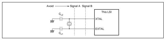
Figure 4.5 Cautions for Oscillator Circuit System Board Design
