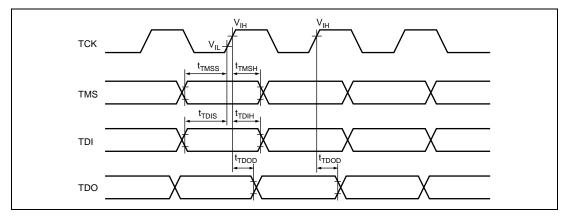
Figure 26.26 H-UDI Input/Output Timing
