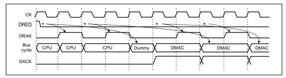
Figure 10.21 Burst Mode, Single Address and Level Detection (Normal Operation)
