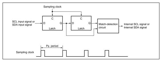
Figure 14.13 A Block Diagram of the Noise Canceller
