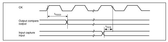
Figure 26.15 MTU Input/Output timing
