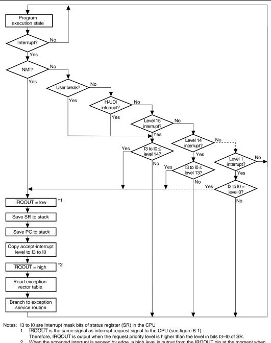
2. When the accepted interrupt is sensed by edge, a high level is output from the IRQOUT pin at the moment when the CPU starts interrupt exception processing instead of instruction execution (namely, before saving SR to stack). However, if the interrupt controller accepts an interrupt with a higher priority than the interrupt just to be accepted and has output an interrupt request to the CPU, the IRQOUT pin holds low level.
