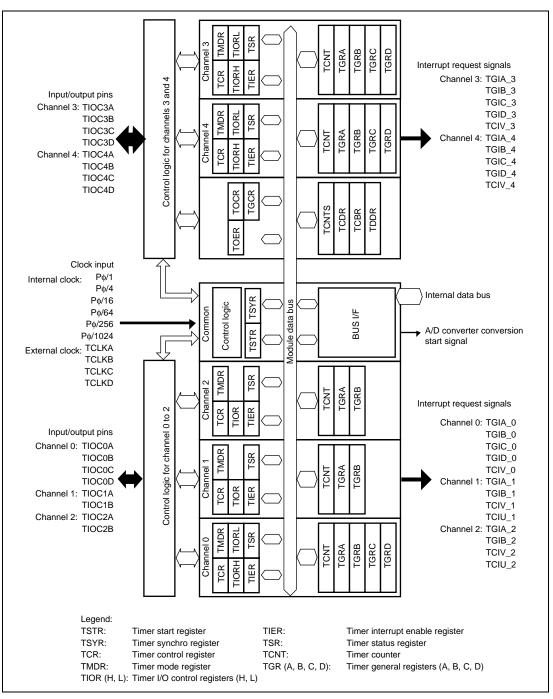
Figure 11.1 Block Diagram of MTU
