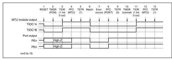
Figure 11.101 Error Occurrence in Phase Counting Mode, Recovery in Normal Mode
