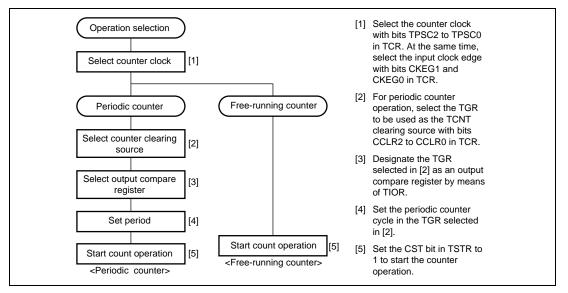
Figure 11.3 Example of Counter Operation Setting Procedure
