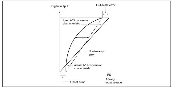
Figure 15.5 Definitions of A/D Conversion Accuracy
