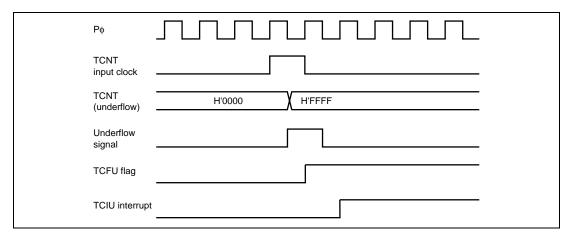
Figure 11.67 TCIU Interrupt Setting Timing
