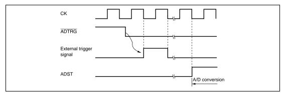
Figure 15.3 External Trigger Input Timing
