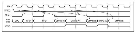
Figure 10.19 Burst Mode, Dual Address and Level Detection (Normal Operation)
