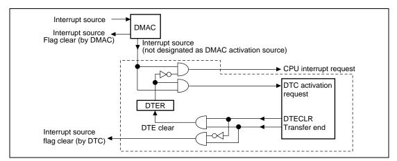
Figure 6.6 Interrupt Control Block Diagram
