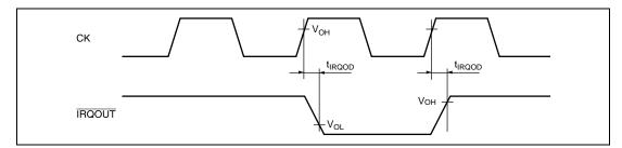
Figure 26.7 Interrupt Signal Output Timing
