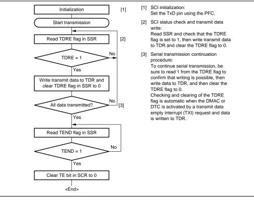
Figure 13.17 Sample Serial Transmission Flowchart
