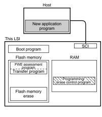
Programming/erase control program transfer When user program mode is entered, user software confirms this fact, executes transfer program in the flash memory, and transfers the programming/erase control program to RAM.
