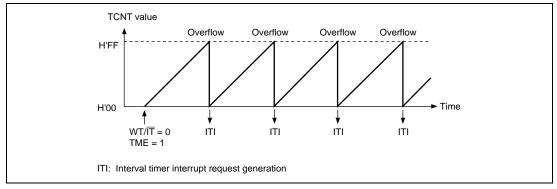
Figure 12.3 Operation in Interval Timer Mode
