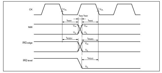
Figure 26.6 Interrupt Signal Input Timing
