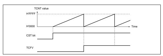
Figure 11.4 illustrates free-running counter operation.
