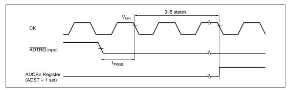
Figure 26.23 External Trigger Input Timing
