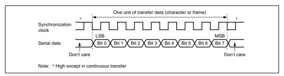
Figure 13.14 Data Format in Clocked Synchronous Communication (For LSB-First)
