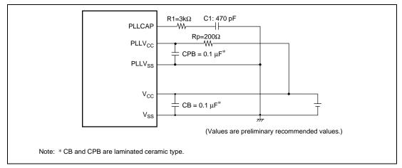
Figure 4.6 Recommended External Circuitry around the PLL
