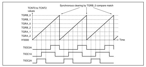
Figure 11.12 Example of Synchronous Operation
