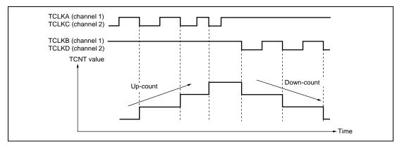
Figure 11.27 Example of Phase Counting Mode 3 Operation
