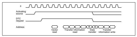
Figure 8.10 DTC Operation Timing Example (Normal Mode)
