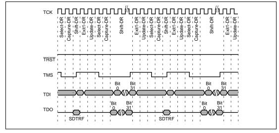
Figure 22.4 Data Input/Output Timing Chart (3)
