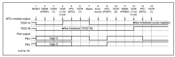
Figure 11.93 Error Occurrence in PWM Mode 1, Recovery in PWM Mode 2
