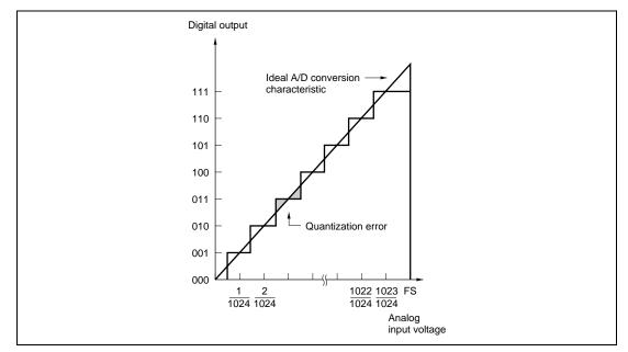
Figure 15.4 Definitions of A/D Conversion Accuracy
