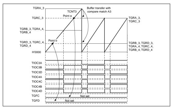
Figure 11.81 Buffer Operation and Compare-Match Flags in Reset Sync PWM Mode
