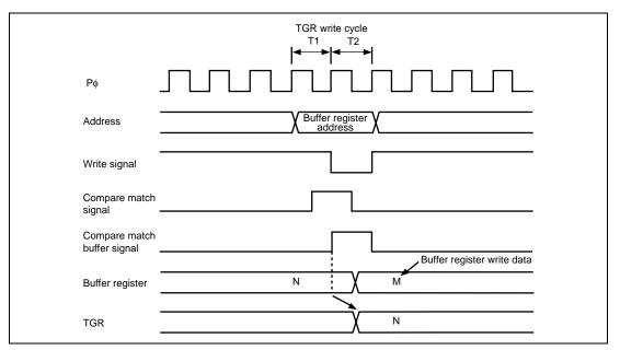
Figure 11.75 Contention between Buffer Register Write and Compare Match (Channels 3 and 4)
