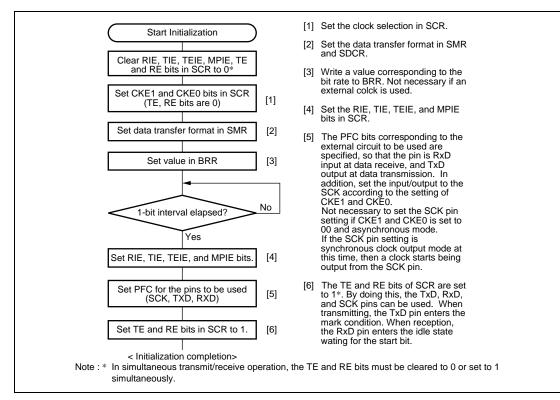
Figure 13.5 Sample SCI Initialization Flowchart
