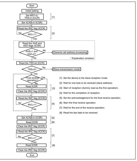
Figure 14.16 Example: Flowchart of Operations in the Slave-Reception Mode
