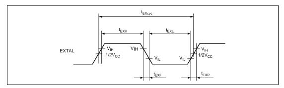
Figure 26.3 EXTAL Clock Input Timing
