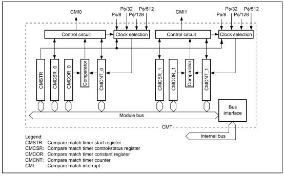
Figure 16.1 CMT Block Diagram
