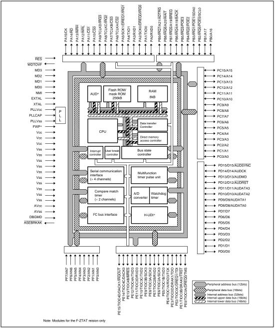
Figure 1.1 Internal Block Diagram of SH7144
