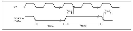
Figure 26.16 MTU Clock Input Timing
