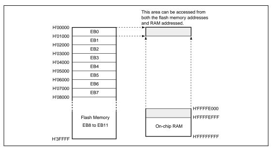
Figure 19.8 Example of RAM Overlap Operation (RAM[2:0] = B'000)
