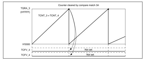
Figure 11.82 Reset Synchronous PWM Mode Overflow Flag
