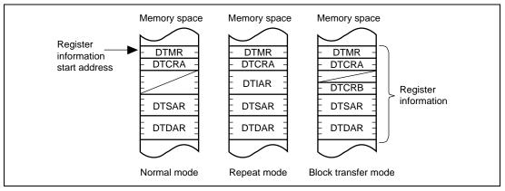
Figure 8.3 DTC Register Information Allocation in Memory Space
