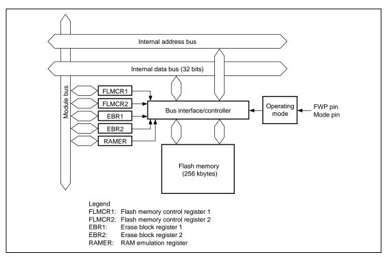
Figure 19.1 Block Diagram of Flash Memory
