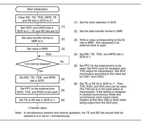
Figure 13.15 Sample SCI Initialization Flowchart
