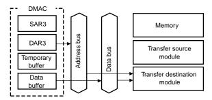
The DAR3 value is taken as the address, and the value in the data buffer is written to the transfer destination module.
