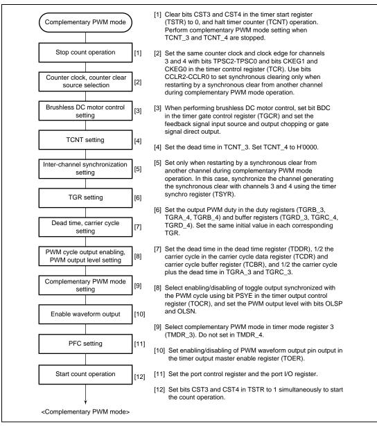
Figure 11.33 Example of Complementary PWM Mode Setting Procedure
