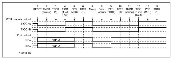
Figure 11.85 Error Occurrence in Normal Mode, Recovery in Normal Mode
