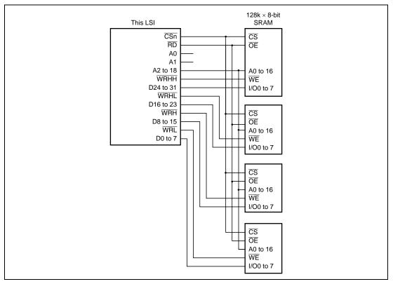
Figure 9.15 Example of 32-bit Data Bus Width SRAM Connection (only for SH7145)
