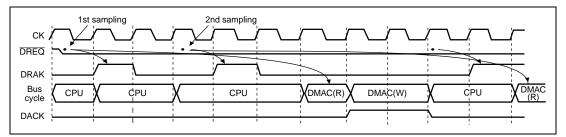
Figure 10.15 Cycle Steal, Dual Address and Level Detection (Normal Operation)
