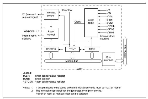
Figure 12.1 Block Diagram of WDT
