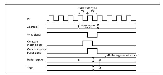
Figure 11.74 Contention between Buffer Register Write and Compare Match (Channel 0)
