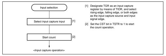
Figure 11.9 Example of Input Capture Operation Setting Procedure
