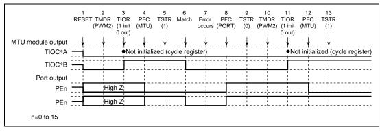
Figure 11.99 Error Occurrence in PWM Mode 2, Recovery in PWM Mode 2
