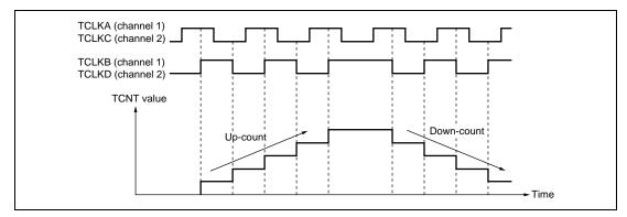
Figure 11.28 Example of Phase Counting Mode 4 Operation
