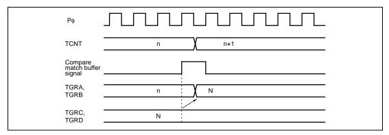
Figure 11.62 Buffer Operation Timing (Compare Match)
