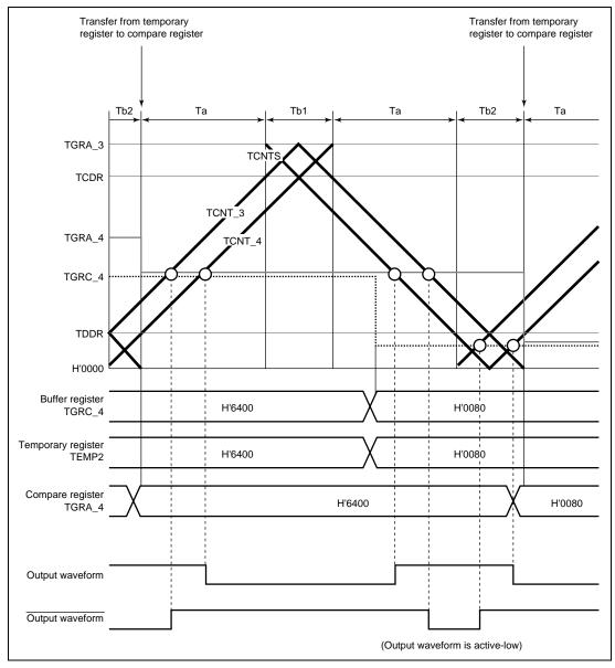
Figure 11.35 Example of Complementary PWM Mode Operation
