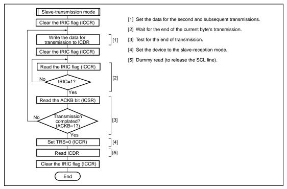
Figure 14.17 Example: Flowchart of Operations in the Slave-Transmission Mode
