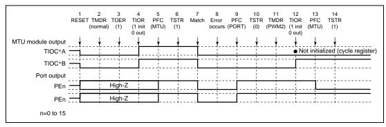
Figure 11.87 Error Occurrence in Normal Mode, Recovery in PWM Mode 2
