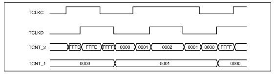
Figure 11.19 Example of Cascaded Operation
