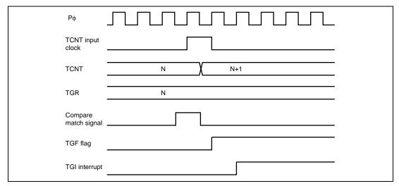
Figure 11.64 TGI Interrupt Timing (Compare Match)
