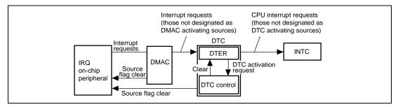
Figure 8.2 Activating Source Control Block Diagram
