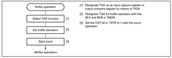
Figure 11.15 Example of Buffer Operation Setting Procedure
