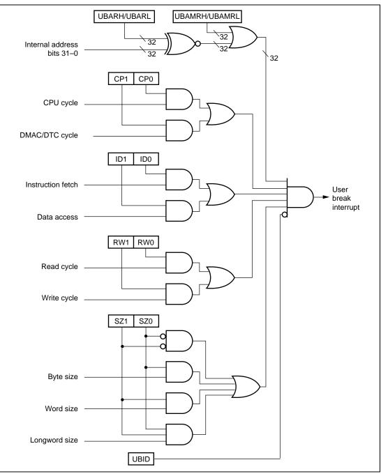
Figure 7.2 Break Condition Determination Method
