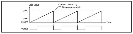
Figure 11.21 Example of PWM Mode Operation (1)
