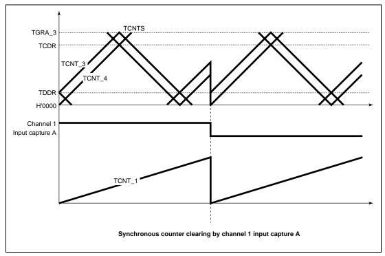
Figure 11.49 Counter Clearing Synchronized with Another Channel
