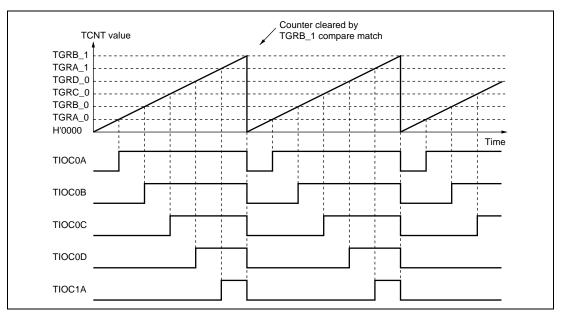
Figure 11.22 Example of PWM Mode Operation (2)
