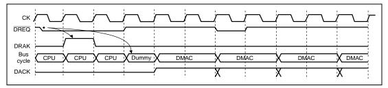
Figure 10.23 Burst Mode, Single Address and Edge Detection
