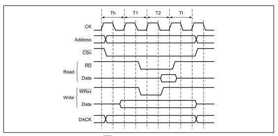
Figure 9.6 CS Assert Period Extension Function
