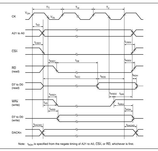
Figure 26.10 Basic Cycle (One Software Wait)
