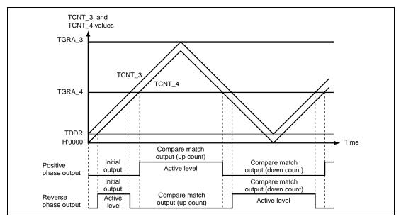
Figure 11.2 Complementary PWM Mode Output Level Example
