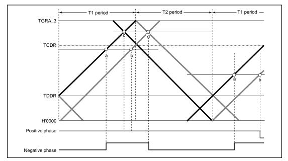
Figure 11.41 Example of Complementary PWM Mode Waveform Output (2)
