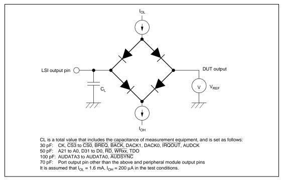
Figure 26.1 Output Load Circuit
