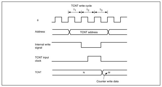
Figure 12.8 Contention between TCNT Write and Increment
