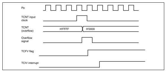
Figure 11.66 TCIV Interrupt Setting Timing
