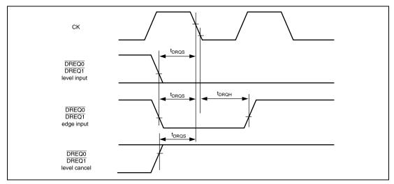
Figure 26.12 DREQ0, DREQ1 Input Timing (1)
