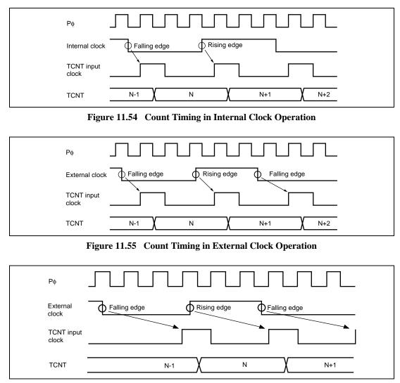
Figure 11.56 Count Timing in External Clock Operation (Phase Counting Mode)
