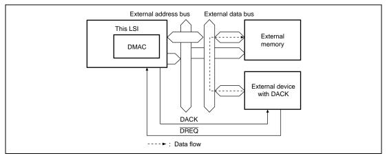
Figure 10.4 Data Flow in Single Address Mode
