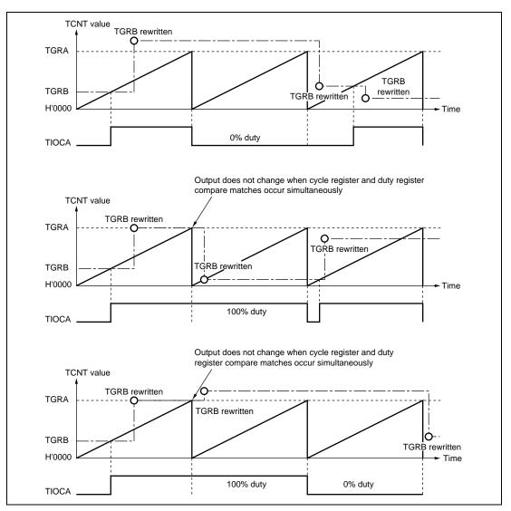
Figure 11.23 shows examples of PWM waveform output with 0% duty and 100% duty in PWM mode.
