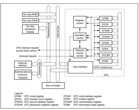
Figure 8.1 Block Diagram of DTC
