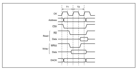
Figure 9.3 Basic Timing of External Space Access
