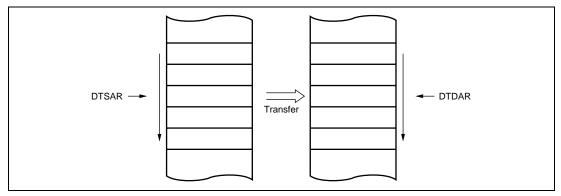
Figure 8.6 Memory Mapping in Normal Mode
