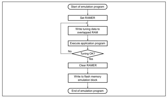
Figure 19.7 Flowchart for Flash Memory Emulation in RAM
