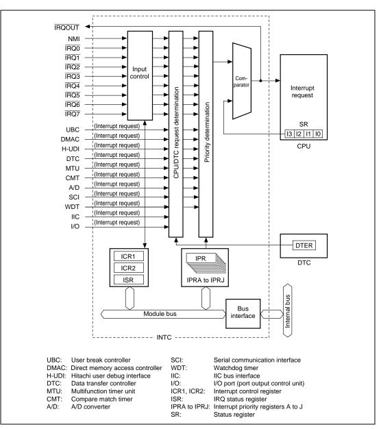
Figure 6.1 INTC Block Diagram
