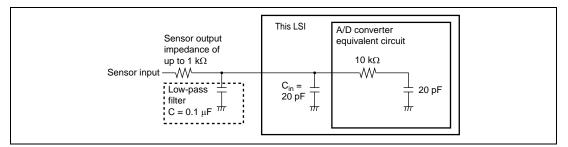
Figure 15.6 Example of Analog Input Circuit
