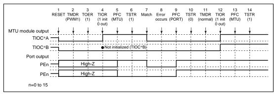
Figure 11.91 Error Occurrence in PWM Mode 1, Recovery in Normal Mode
