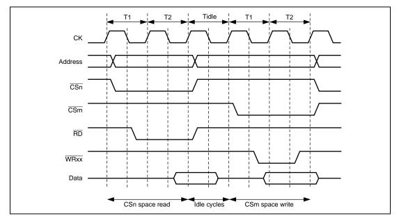
Figure 9.7 Example of Idle Cycle Insertion
