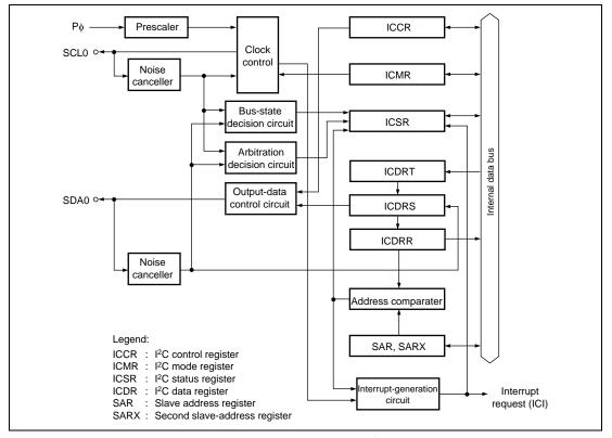
Figure 14.1 A Block Diagram of the I<sup>2</sup>C Bus Interface
