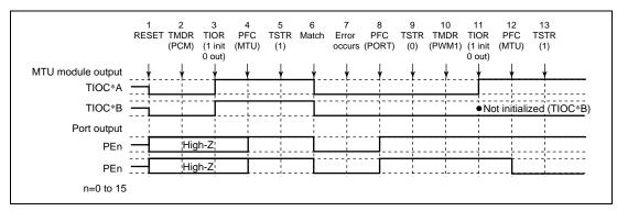
Figure 11.102 Error Occurrence in Phase Counting Mode, Recovery in PWM Mode 1
