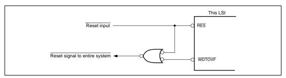
Figure 12.9 Example of System Reset Circuit Using WDTOVF Signal
