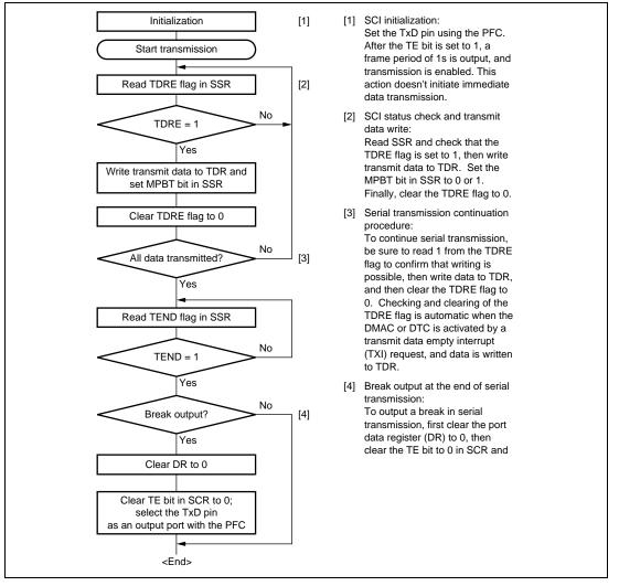
Figure 13.11 Sample Multiprocessor Serial Transmission Flowchart
