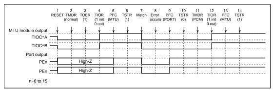
Figure 11.88 Error Occurrence in Normal Mode, Recovery in Phase Counting Mode
