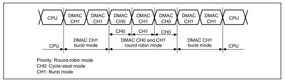
Figure 10.13 Bus Handling when Multiple Channels Are Operating
