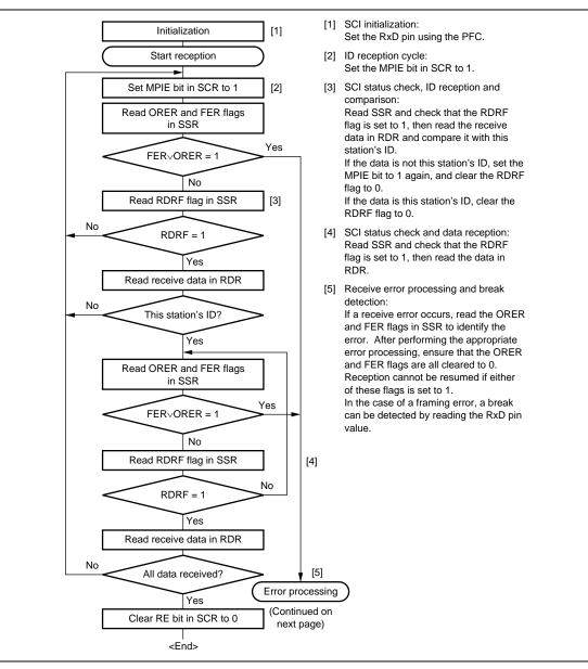
Figure 13.13 Sample Multiprocessor Serial Reception Flowchart (1)
