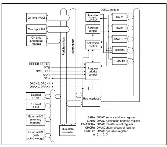
Figure 10.1 DMAC Block Diagram
