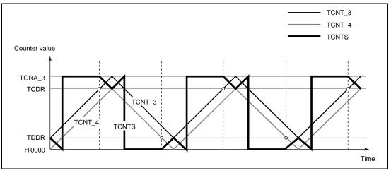
Figure 11.34 Complementary PWM Mode Counter Operation
