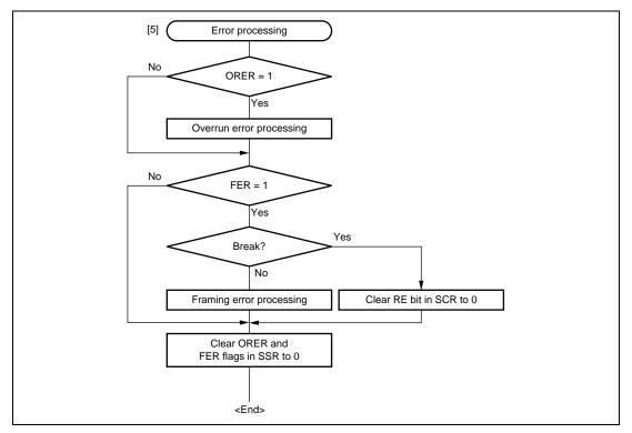
Figure 13.13 Sample Multiprocessor Serial Reception Flowchart (2)
