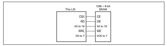
Figure 9.13 Example of 8-bit Data Bus Width SRAM Connection
