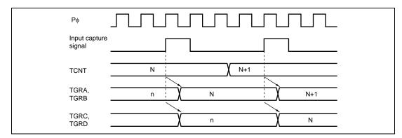
Figure 11.63 Buffer Operation Timing (Input Capture)
