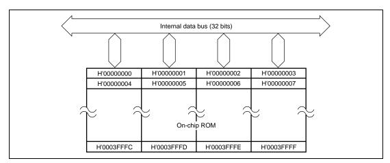
Figure 20.1 Mask ROM Block Diagram
