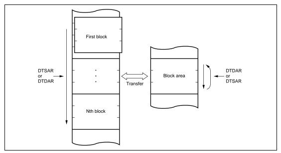
Figure 8.8 Memory Mapping in Block Transfer Mode
