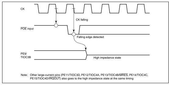
Figure 11.117 shows an example of timing from  $\overline{POE}$  input to high impedance of pin.
