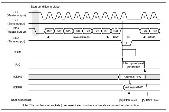
Figure 14.9 An Example of the Timing of Operations in Slave-Reception Mode (1) (MLS = ACKB = 0)
