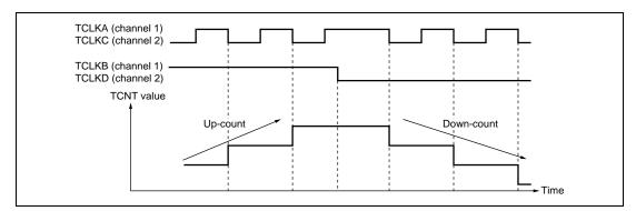
Figure 11.26 Example of Phase Counting Mode 2 Operation
