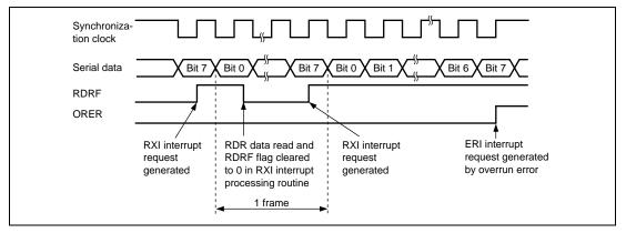
Figure 13.18 Example of SCI Operation in Reception
