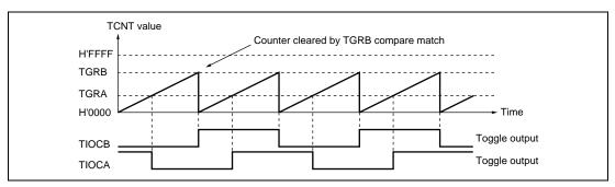
Figure 11.8 Example of Toggle Output Operation
