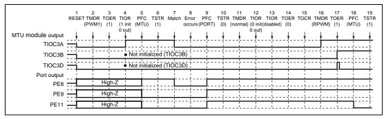
Figure 11.96 Error Occurrence in PWM Mode 1, Recovery in Reset-Synchronous PWM Mode
