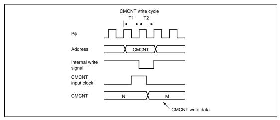
Figure 16.7 CMCNT Word Write and Increment Contention
