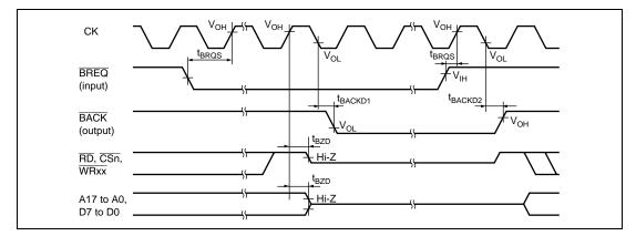
Figure 26.8 Bus Release Timing
