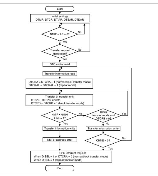
Figure 8.5 DTC Operation Flowchart
