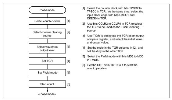
Figure 11.20 Example of PWM Mode Setting Procedure
