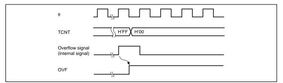
Figure 12.4 Timing of Setting OVF
