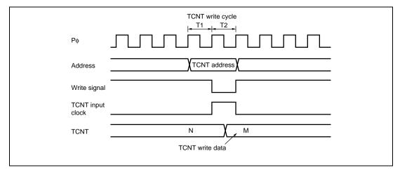
Figure 11.72 Contention between TCNT Write and Increment Operations
