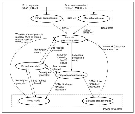
Figure 2.4 Transitions between Processing States
