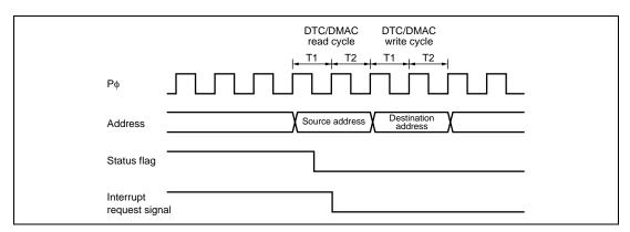
Figure 11.69 Timing for Status Flag Clearing by DTC/DMAC Activation
