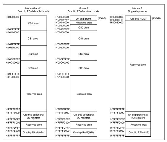
Figure 3.1 The Address Map for Each Operating Mode
