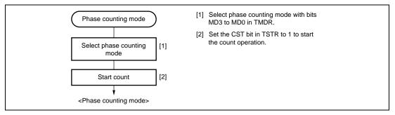
Figure 11.24 Example of Phase Counting Mode Setting Procedure
