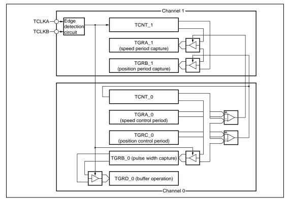
Figure 11.29 Phase Counting Mode Application Example
