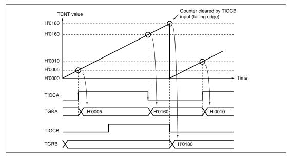
Figure 11.10 Example of Input Capture Operation
