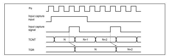
Figure 11.59 Input Capture Input Signal Timing
