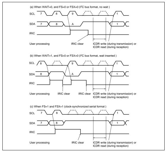
Figure 14.12 IRIC-Set Timing and the Control of SCL
