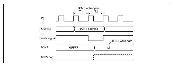
Figure 11.84 Contention between TCNT Write and Overflow
