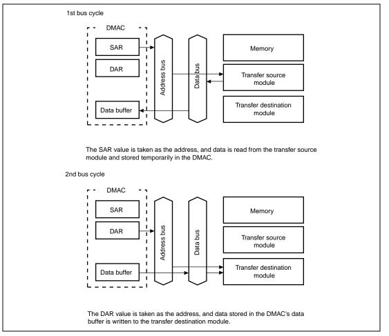
Figure 10.6 Direct Address Operation during Dual Address Mode
