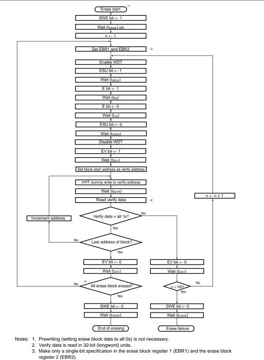
4. Erasing is performed in block units. To erase multiple blocks, each block must be erased in turn.
