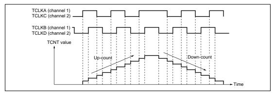
Figure 11.25 Example of Phase Counting Mode 1 Operation
