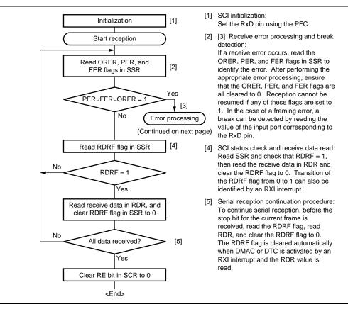
Figure 13.9 Sample Serial Reception Data Flowchart (1)
