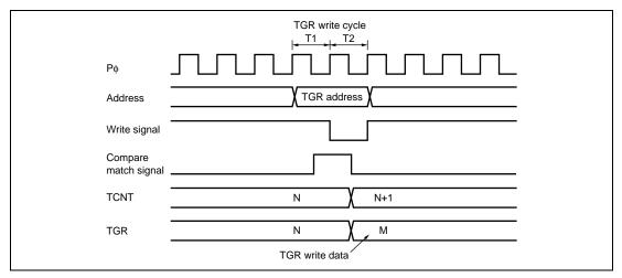
Figure 11.73 Contention between TGR Write and Compare Match
