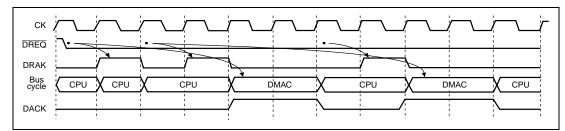
Figure 10.17 Cycle Steal, Single Address and Level Detection (Normal Operation)
