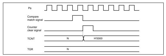
Figure 11.60 Counter Clear Timing (Compare Match)
