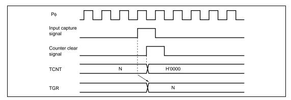
Figure 11.61 Counter Clear Timing (Input Capture)
