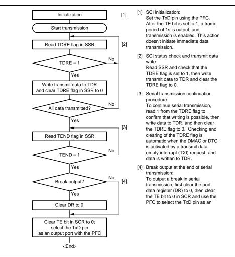
Figure 13.7 Sample Serial Transmission Flowchart
