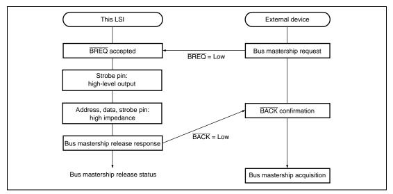
Figure 9.9 Bus Mastership Release Procedure
