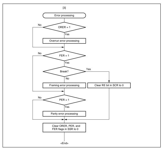
Figure 13.9 Sample Serial Reception Data Flowchart (2)
