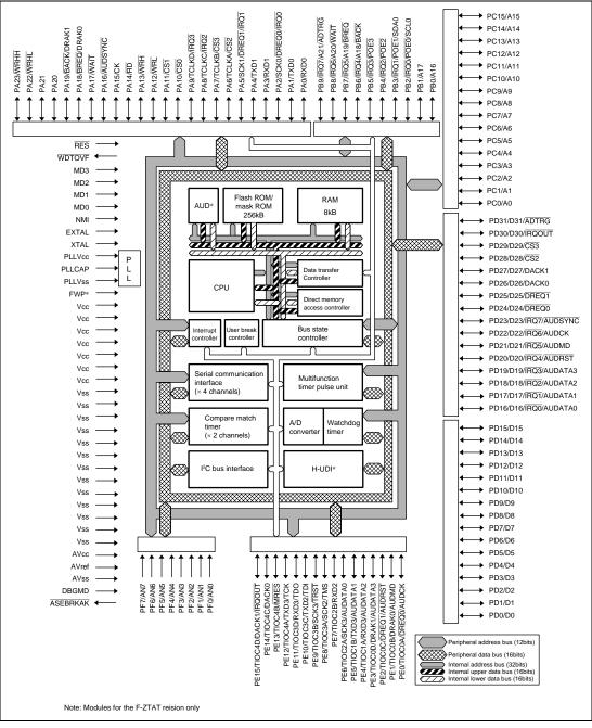
Figure 1.2 Block Diagram of SH7145
