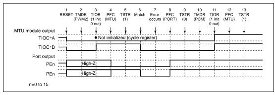
Figure 11.100 Error Occurrence in PWM Mode 2, Recovery in Phase Counting Mode
