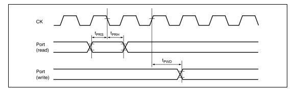
Figure 26.17 I/O Port Input/Output timing
