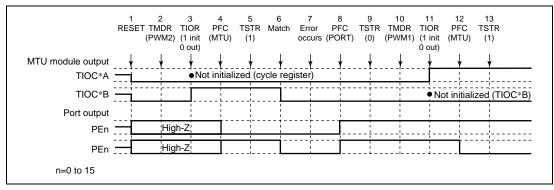
Figure 11.98 Error Occurrence in PWM Mode 2, Recovery in PWM Mode 1
