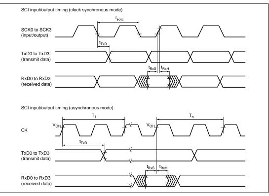
Figure 26.20 SCI Input/Output Timing
