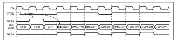
Figure 10.22 Burst Mode, Dual Address and Edge Detection
