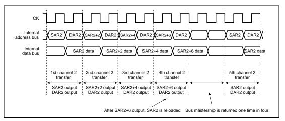
Figure 10.25 Source Address Reload Function Timing Chart
