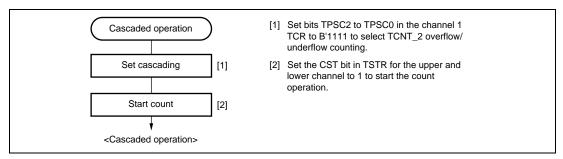
Figure 11.18 Cascaded Operation Setting Procedure
