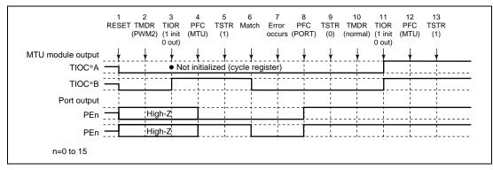
Figure 11.97 Error Occurrence in PWM Mode 2, Recovery in Normal Mode
