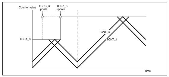
Figure 11.36 Example of PWM Cycle Updating
