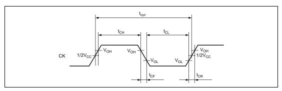
Figure 26.2 System Clock Timing
