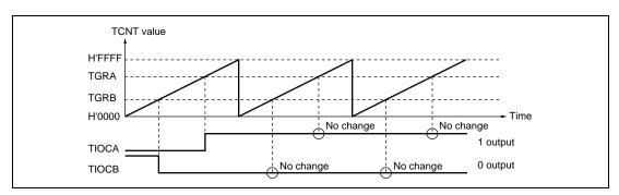
Figure 11.7 Example of 0 Output/1 Output Operation
