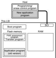
Flash memory initialization The programming/erase program in RAM is executed, and the flash memory is initialized (to H'FF). Erasing can be performed in block units, but not in byte units.
