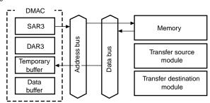
The SAR3 value is taken as the address, memory data is read, and the value is stored in the temporary buffer. Since the value read at this time is used as the address, it must be 32 bits. When external connection data bus is 16 bits, two bus cycles are required.
