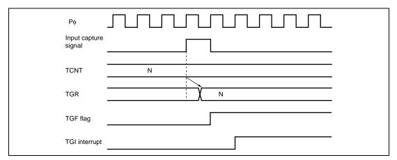
Figure 11.65 TGI Interrupt Timing (Input Capture)
