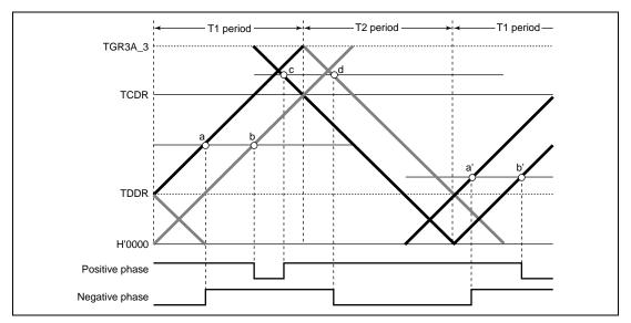
Figure 11.40 Example of Complementary PWM Mode Waveform Output (1)
