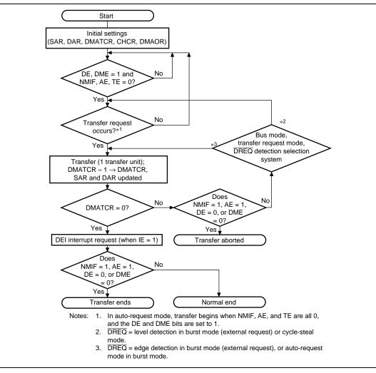
Figure 10.2 DMAC Transfer Flowchart
