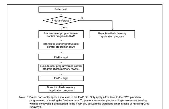
Figure 19.6 Programming/Erasing Flowchart Example in User Program Mode
