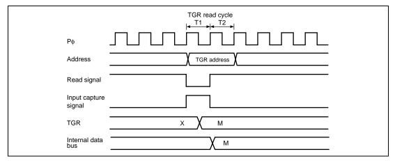
Figure 11.76 Contention between TGR Read and Input Capture
