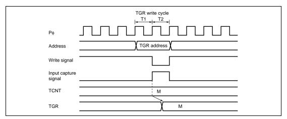
Figure 11.77 Contention between TGR Write and Input Capture
