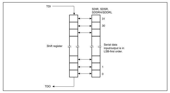
Figure 22.5 Serial Data Input/Output
