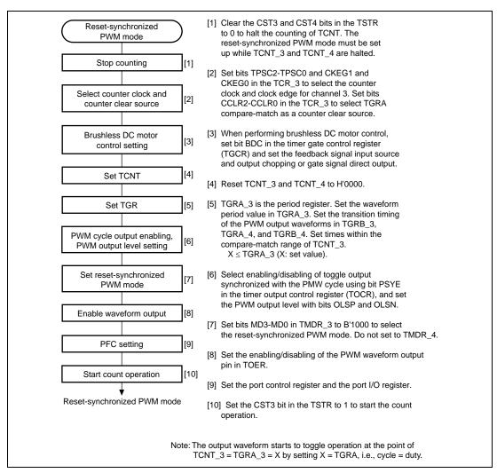
Figure 11.30 Procedure for Selecting the Reset-Synchronized PWM Mode
