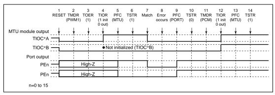
Figure 11.94 Error Occurrence in PWM Mode 1, Recovery in Phase Counting Mode
