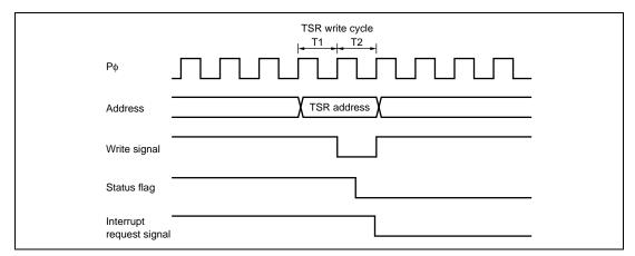
Figure 11.68 Timing for Status Flag Clearing by the CPU
