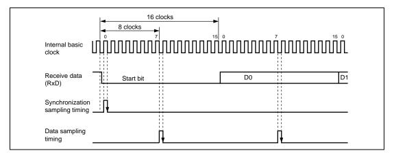
Figure 13.3 Receive Data Sampling Timing in Asynchronous Mode
