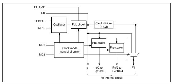
Figure 4.1 Block Diagram of the Clock Pulse Generator
