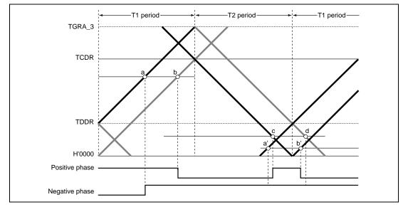
Figure 11.42 Example of Complementary PWM Mode Waveform Output (3)
