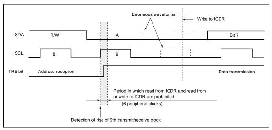
Figure 14.21 Scheme of Slave Transmit Operation
