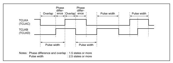
Figure 11.70 Phase Difference, Overlap, and Pulse Width in Phase Counting Mode
