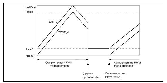
Figure 11.80 Counter Value during Complementary PWM Mode Stop
