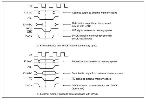
Figure 10.5 Example of DMA Transfer Timing in the Single Address Mode
