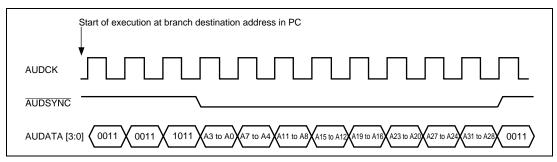
Figure 23.2 Example of Data Output (32-Bit Output)
