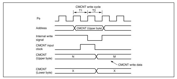
Figure 16.8 CMCNT Byte Write and Increment Contention
