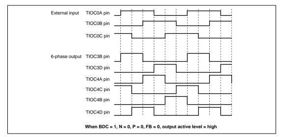
Figure 11.50 Example of Output Phase Switching by External Input (1)
