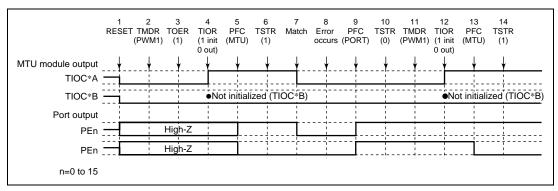
Figure 11.92 Error Occurrence in PWM Mode 1, Recovery in PWM Mode 1
