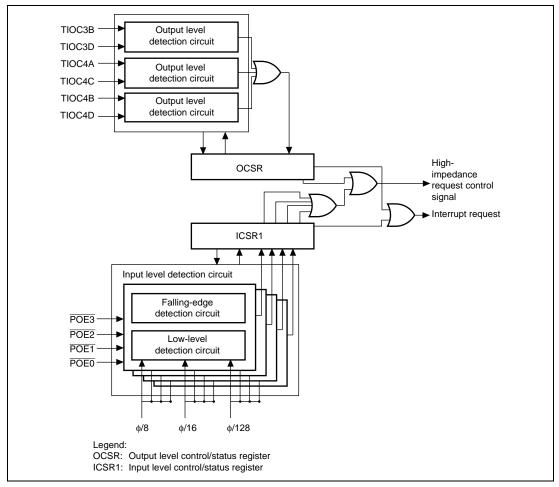
Figure 11.114 POE Block Diagram
