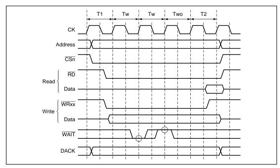
Figure 9.5 Wait State Timing of External Space Access (Two Software Wait States + WAIT Signal Wait State)
