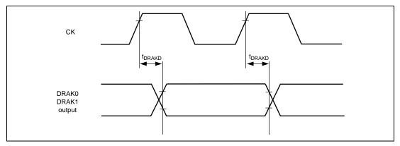
Figure 26.14 DRAK Output Delay Time
