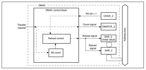
Figure 10.24 Source Address Reload Function
