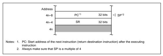
Figure 6.4 Stack after Interrupt Exception Processing
