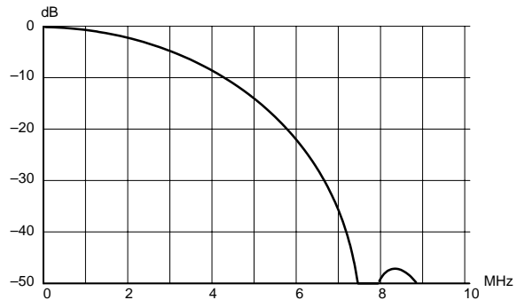
Fig. 2-20: Frequency response of the chroma interpolation filter
