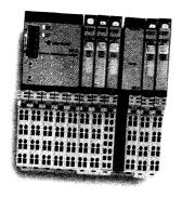
The second DeviceNet communication interface option integrates 16 digital I/O points of 120V ac or 24V dc configurations into a single package (1734D or POINT Block I/O). Outputs are available with solid state, triac or relays. As with the adapter, this solution provides physical address selection and may be expanded with any POINT I/O modules, however each additional POINT I/O module on this interface is seen as an individual node on the DeviceNet communication network.
