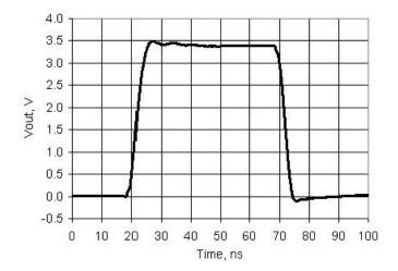
Figure 11-16. GPIO Output Rise and Fall Times, Slow Strong Mode,  $V_{\mbox{DDIO}}$  = 3.3 V, 25 pF Load
