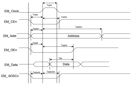
Figure 11-53. Synchronous Read Cycle Timing
