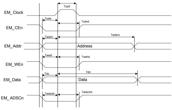
Figure 11-54. Synchronous Write Cycle Timing
