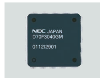
176-pin plastic LQFP 0.5 mm pitch, 24 × 24 mm, 1.4 mm thick
