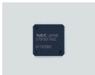
100-pin plastic LQFP 0.5 mm pitch, 14 × 14 mm, 1.4 mm thick
