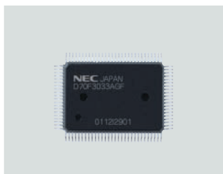
100-pin plastic QFP 0.65 mm pitch, 14 × 20 mm, 3.0 mm thick
