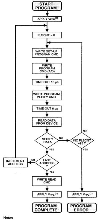
(1) See DC Characteristics for the value of  $V_{\rm pph}$ . The  $V_{\rm pp}$ supply can be hard wired to the device or switchable. When  $V_{PP}$  is switched,  $V_{PPL}$  may be GND, NC with a resistor tied to GND or less than V<sub>cc</sub>+2.0V
