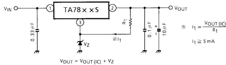
(b) Voltage boost by use of resistor
