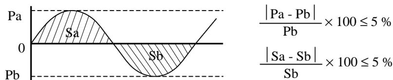
Pa: Supply voltage/current peak for positive, Pb: Supply voltage/current peak for negative
