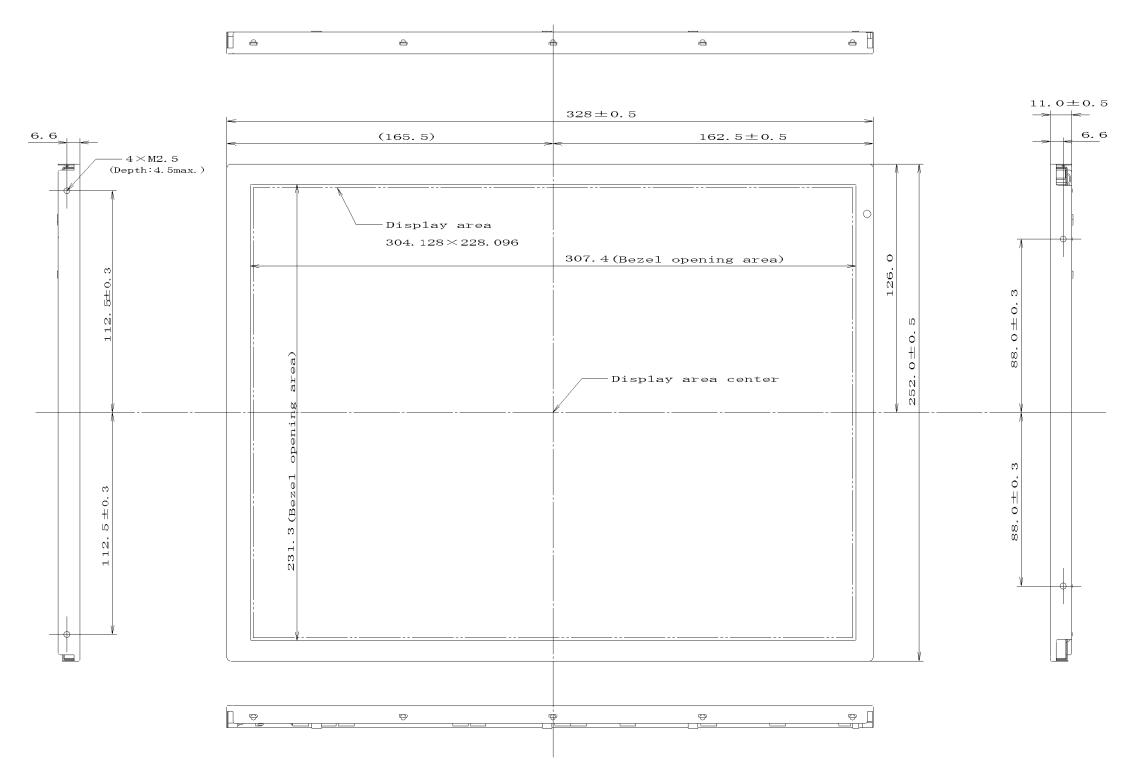
Note1: Not shown tolerances of the dimensions are  $\pm 0.5$ mm.
