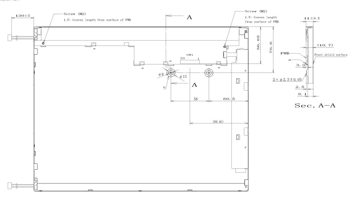
Note1: Not shown tolerances of the dimensions are  $\pm 0.5$ mm.
