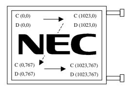
Note1: Meaning of C(X, Y) and D(X, Y)
