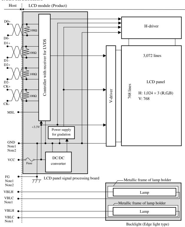
Note1: Connections between GND (Signal ground), FG (Frame ground) and VBLC (Lamp low voltage terminal) in the product
