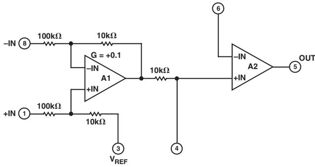
Figure 3. Simplified Schematic
