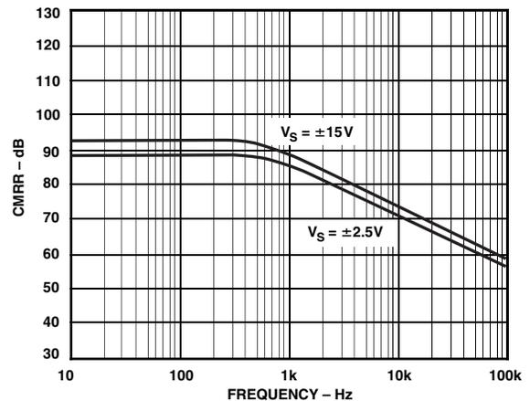
Figure 1. CMRR vs. Frequency of the AD628
