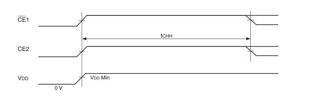
Note: The tchh specifies after Vdd reaches specified minimum level and applicable both  $\overline{\text{CE}}1$  and CE2. If transition time of Vdd (from 0 V to Vdd Min) is longer than 50 ms, POWER-UP Timing #1 must be applied.
