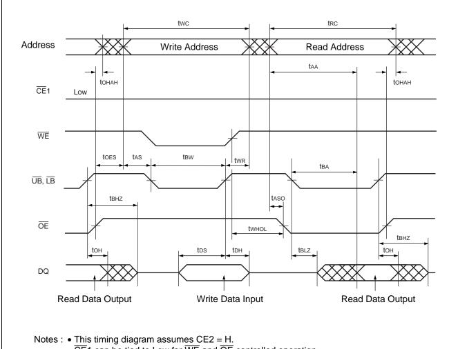
•  $\overline{\text{CE}}$ 1 can be tied to Low for  $\overline{\text{WE}}$  and  $\overline{\text{OE}}$  controlled operation.
