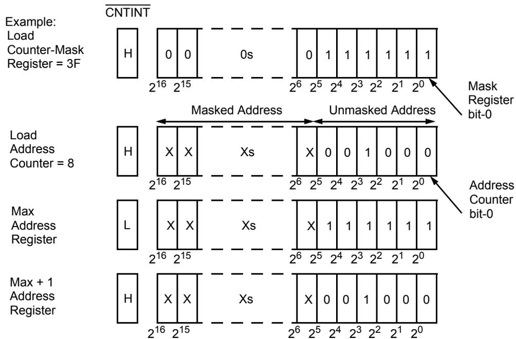
**Figure 2. Programmable Counter-Mask Register Operation**<sup>[1, 20]</sup>
