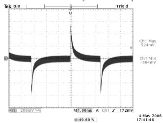
**Photo 10:** Transient Response – 0.25A/us Vin=24 V, Iout = 0.25 to 1 A (25% to 100%)
