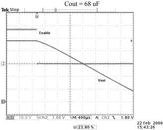
**Photo 6:** Turn Off by Enable at 24 V Cout = 68 uF
