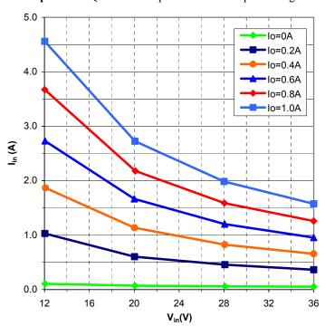
**Graph 4:** MPQ24S48-50 Power Dissipation vs. Input Voltage
