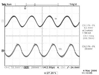
**Photo 2:** Input Ripple Voltage and Current Vin=24 V, Iout = 1 A
