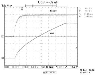
**Photo 5:** Turn On by Enable at 24 V Cout = 68 uF
