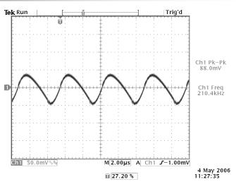
Photo 8: Output Ripple and Noise (20 MHz BW)
