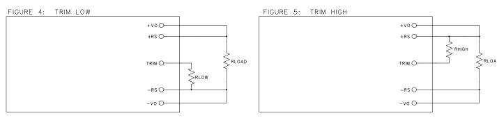
NOTE 1: CONNECT TRIM RESISTOR AS CLOSE TO CONVERTER PINS AS POSSIBLE
