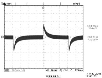
**Photo 9:** Transient Response – 0.025A/us Vin=24 V, Iout = 0.25 to 1 A (25% to 100%)
