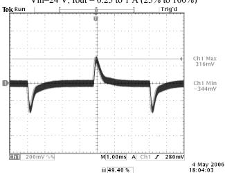
**Photo 10:** Transient Response – 0.025A/us Vin=24 V, Iout = 0.25 to 1 A (25% to 100%) With a 68 uF Electrolytic across the Output
