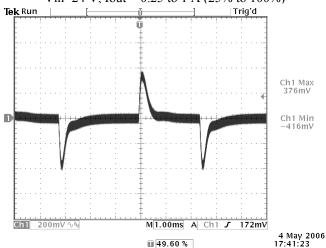
**Photo 11:** Transient Response -0.25A/us Vin=24 V, Iout = 0.25 to 1 A (25% to 100%) With a 68 uF Electrolytic across the Output
