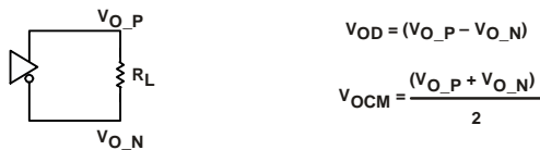
Figure 12. Link Ports—Transmit Electrical Characteristics
