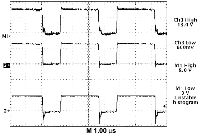
Channel 3 = V GATE M1 = V GATE - 5.0 V IN Channel 2 – Inductor Switching Node
