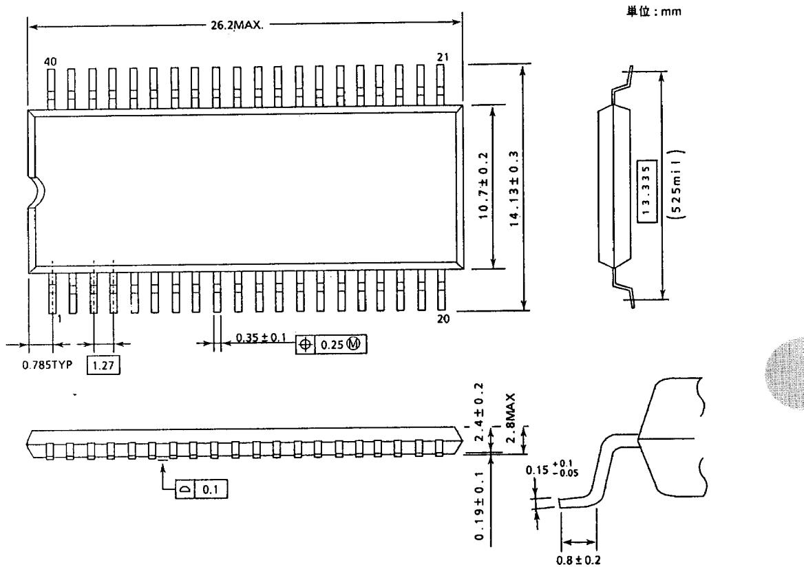
Note: Package width and length do not include mold protrusion, allowable mold protrusion is 0.15mm.
