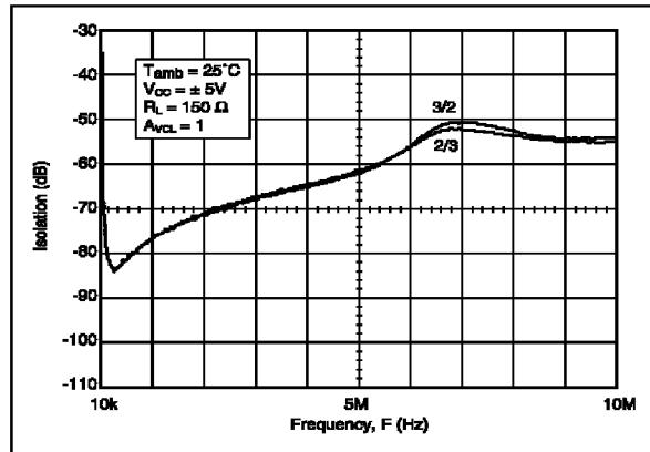
**INPUT/OUTPUT ISOLATION IN STANDBY MODE (SO16 PACKAGE)**
