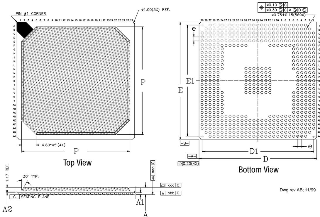
Figure 23. 569-Ball Plastic Ball Grid Array (PBGA) Package
