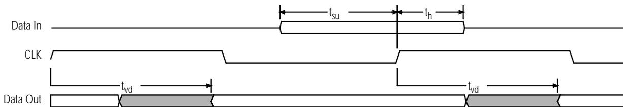
Figure 18. Setup, Hold, and Valid Delay Timings
