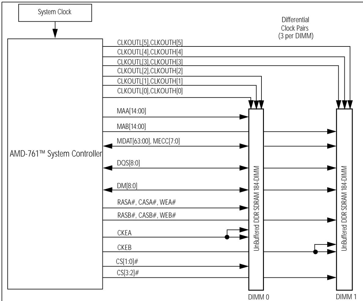
Figure 4. AMD-761™ System Controller Connection to Unbuffered DIMMs
