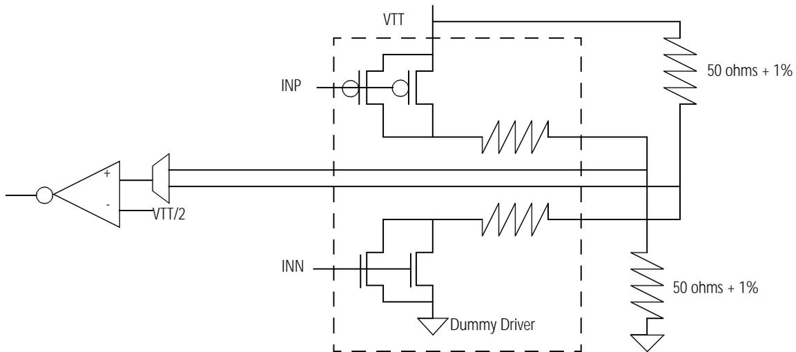
**Figure 3. Dummy Load with External Compensation Resistors**
