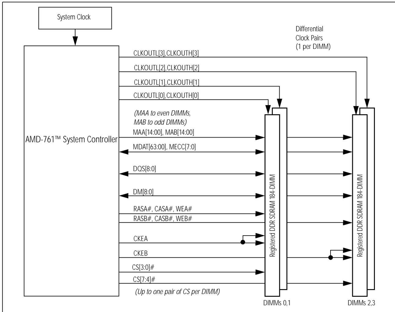
Figure 5. AMD-761™ System Controller Connection to Registered DIMMs
