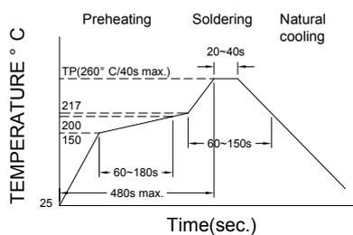
Figure 1. Re-flow Soldering
