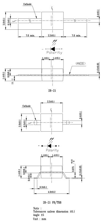
**Note:** Tolerances Unless Dimension is  $\pm 0.1$ mm, Unit = mm
