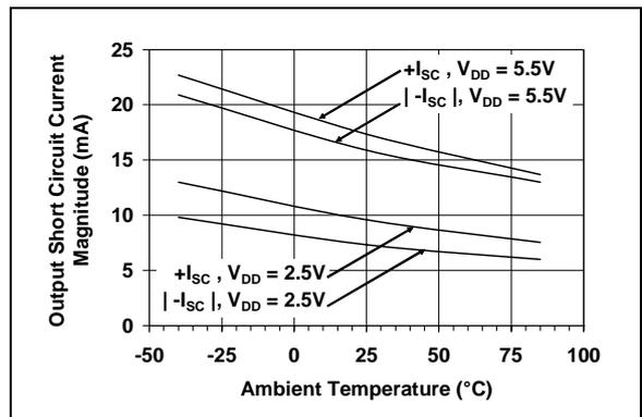
**FIGURE 2-24:** Output Short Circuit Current Magnitude vs. Ambient Temperature.
