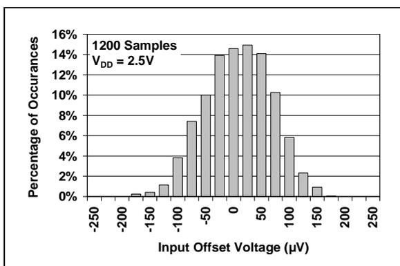
**FIGURE 2-2:** Input Offset Voltage at  $V_{DD} = 2.5V$ .
