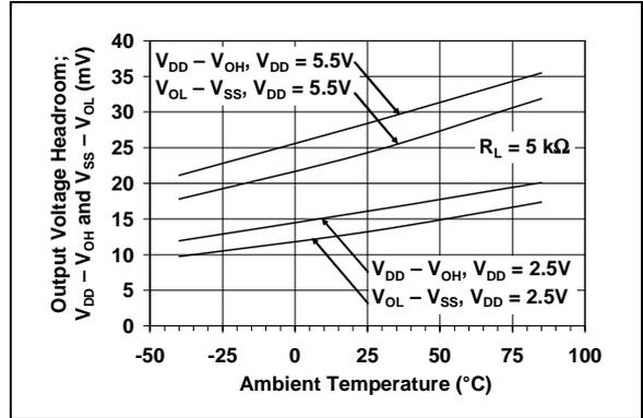
**FIGURE 2-22:** Output Voltage Headroom vs. Ambient Temperature at  $R_L = 5\text{ k}\Omega$ .
