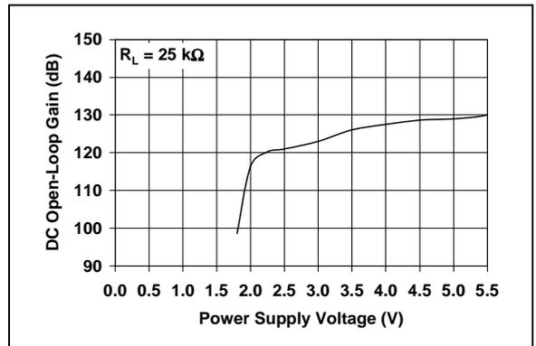
**FIGURE 2-17:** DC Open-Loop Gain vs. Power Supply Voltage.
