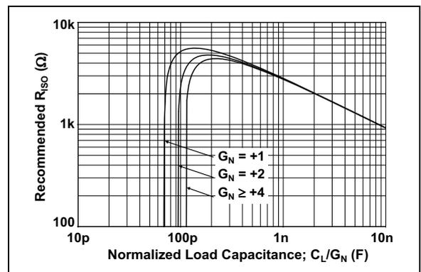
**FIGURE 4-3:** Recommended  $R_{ISO}$  Values for Capacitive Loads.
