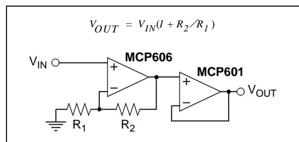
**FIGURE 4-10:** Precision Gain with Good Load Isolation.
