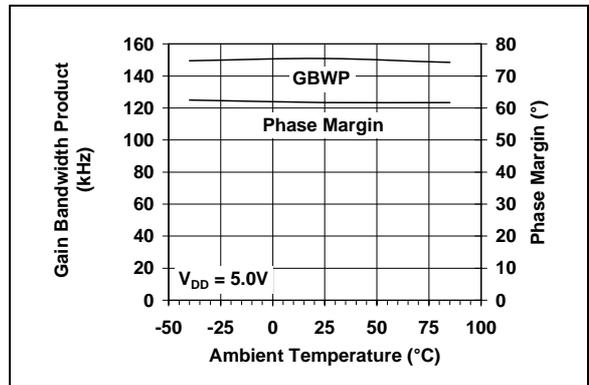
**FIGURE 2-11:** Gain Bandwidth Product, Phase Margin vs. Ambient Temperature.
