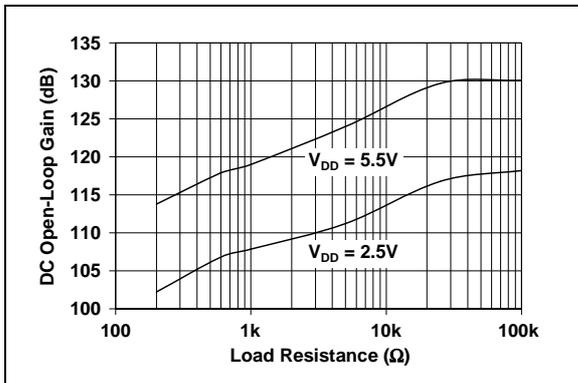
**FIGURE 2-14:** DC Open-Loop Gain vs. Load Resistance.
