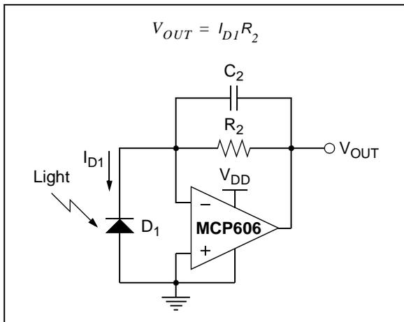
**FIGURE 4-6:** Photodiode (in Photo-voltaic mode) and Transimpedance Amplifier.
