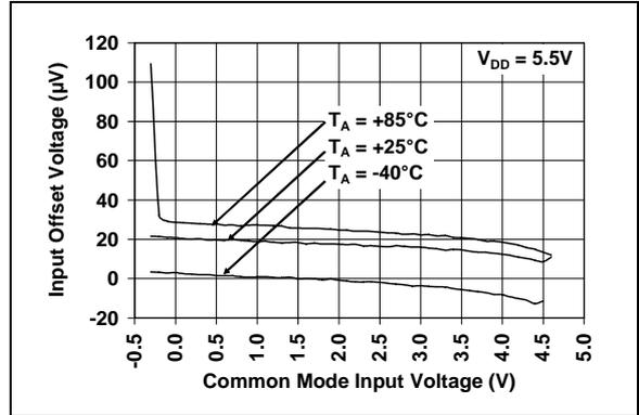
**FIGURE 2-10:** Input Offset Voltage vs. Common Mode Input Voltage.
