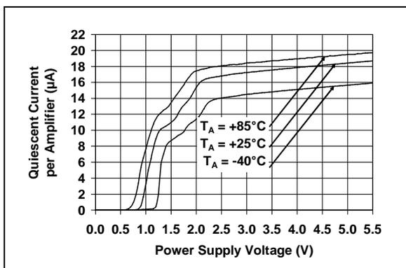
**FIGURE 2-3:** Quiescent Current vs. Power Supply Voltage.
