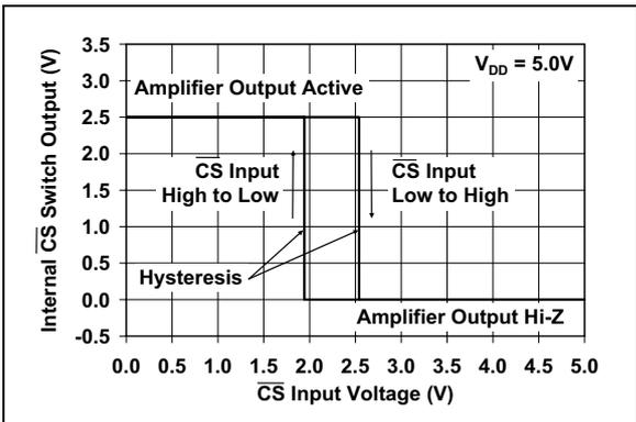
**FIGURE 2-27:** Chip Select ( $\overline{CS}$ ) Hysteresis (MCP608 only).
