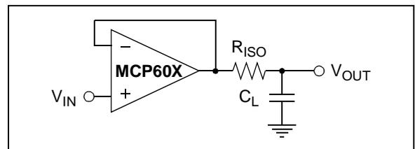
**FIGURE 4-2:** Output Resistor,  $R_{ISO}$  stabilizes large capacitive loads.
