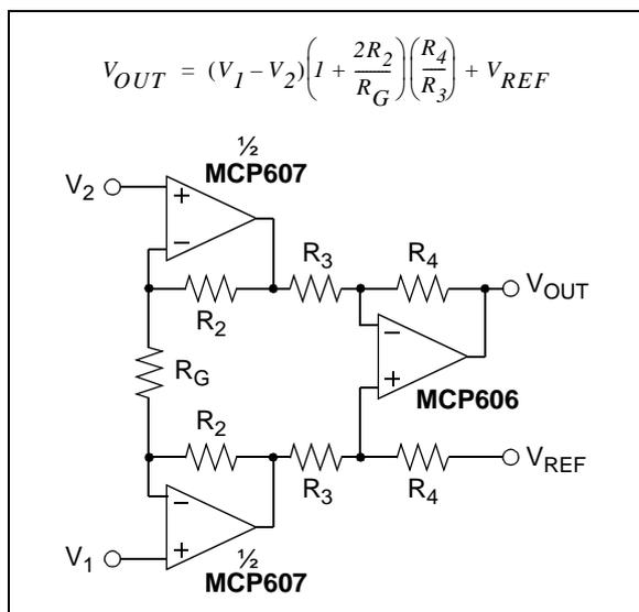
**FIGURE 4-9:** Three op amp Instrumentation Amplifier.
