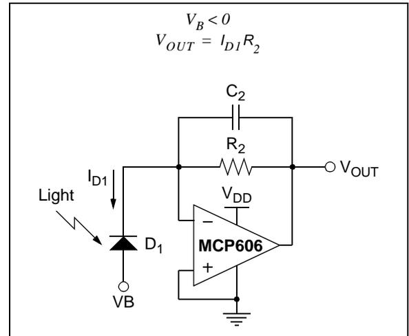
**FIGURE 4-7:** Photodiode (in Photo-conductive mode) and Transimpedance Amplifier.
