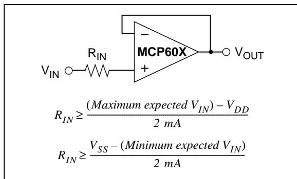
**FIGURE 4-1:** Input Current-Limiting Resistor ( $R_{IN}$ ).
