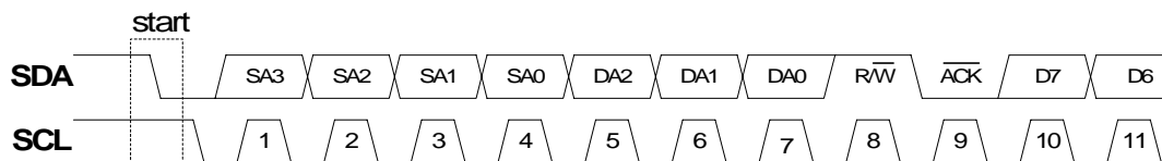
Figure 4-6. Addressing an I 2 C Peripheral
