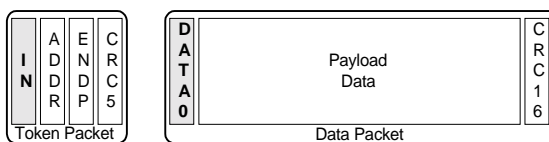
Figure 1-6. An Isochronous Transfer
