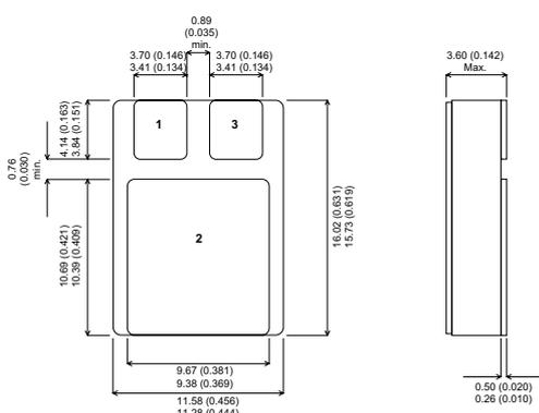
Pin1 - Adjust      Pin 2 - Input      Pin 3 - Output
