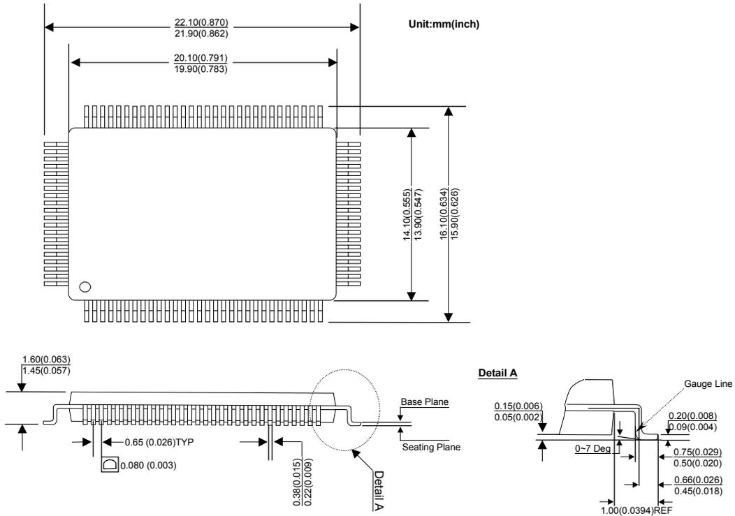
All dimension in mm (inches). Notation is  $\frac{\text{MAX}}{\text{MIN}}$  or typical.
