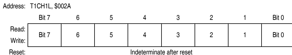
Figure 17-16. TIM Channel 1 Register Low (TCH1L)
