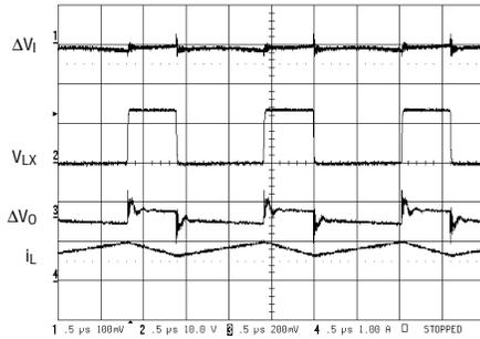
Steady State Operation (inductor discontinuous conduction)
