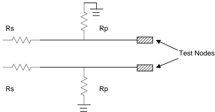
Figure 3. Lumped Test Load Configuration
