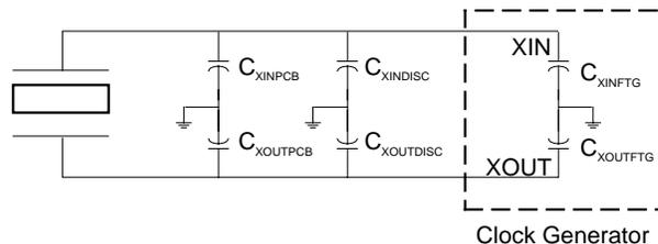
As an example, and using this formula for this datasheet's device, a design that has no discrete loading capacitors (C<sub>DISC</sub>) and each of the crystal to device PCB traces has a capacitance (C<sub>PCB</sub>) to ground of 4pF (typical value) would calculate as:
