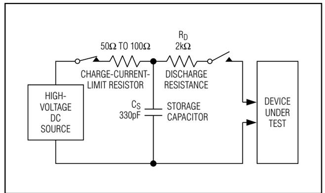
Figure 15. ISO 10605 Contact-Discharge ESD Test Circuit
