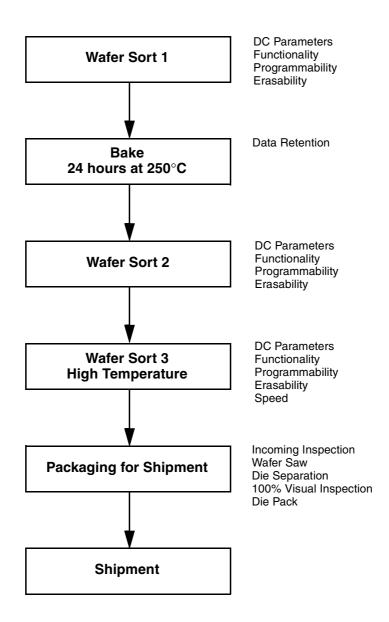
Figure 1. AMD KGD Product Test Flow
